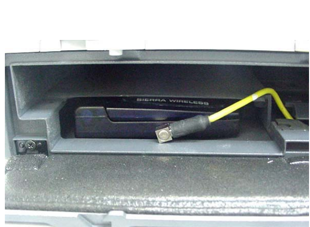
Photograph A.1-6 - CDMA Modem installed in DUT
