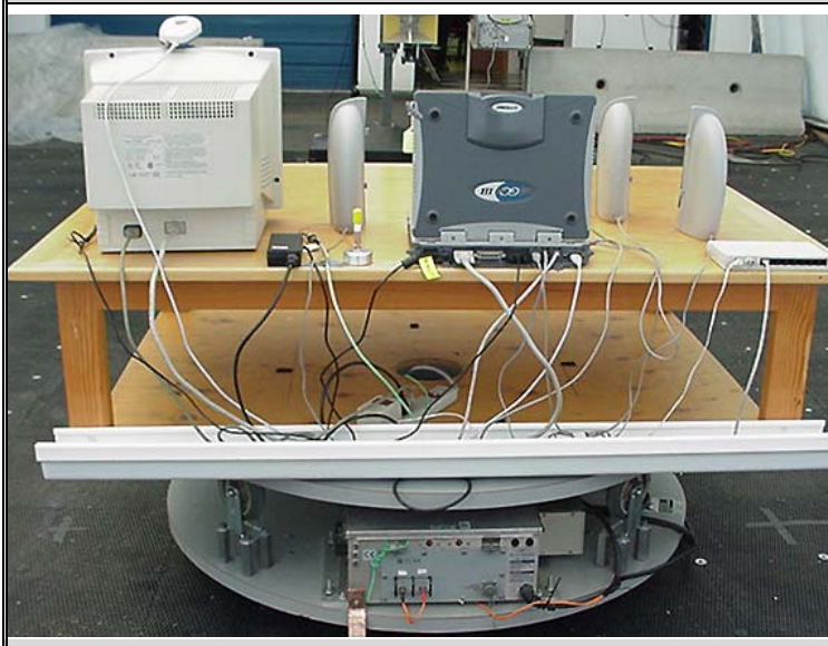
Photograph C.7-5 - Back of Radiated Emissions Setup with attached swivel dipole antenna
