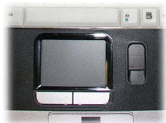
Resistive Touchpad option: works with gloved fingers
