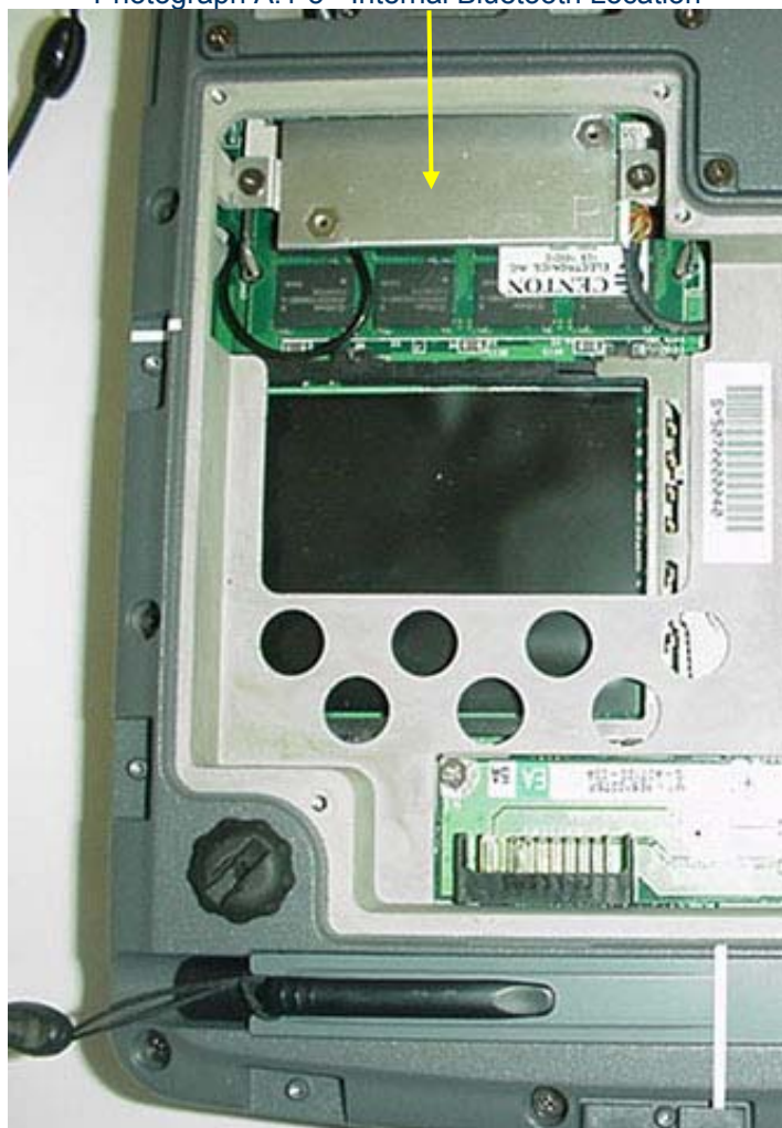
Photograph A.1-5 - Internal Bluetooth Location
