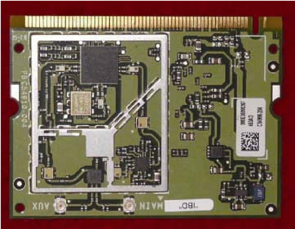
Front with Shielding Removed
