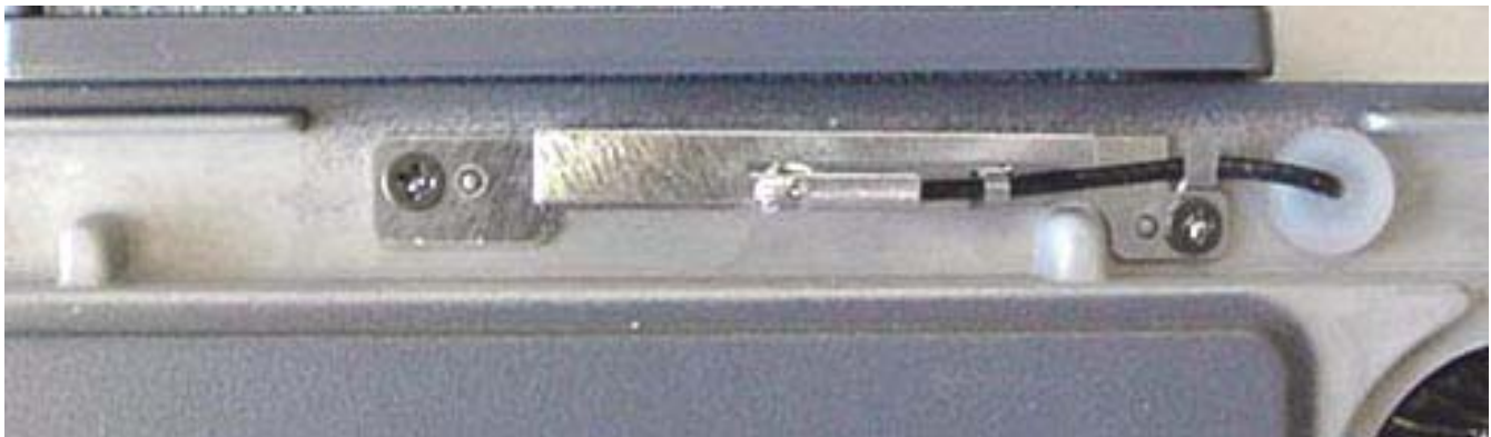
WLAN Antenna 2 (Transmit / Receive)
