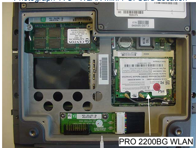
Photograph A-5 - WLAN Mini-PCI Card Location
