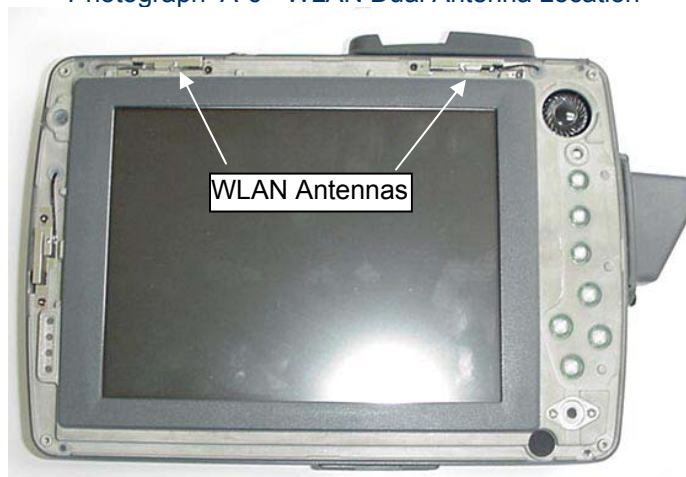
Photograph A-6 - WLAN Dual Antenna Location
