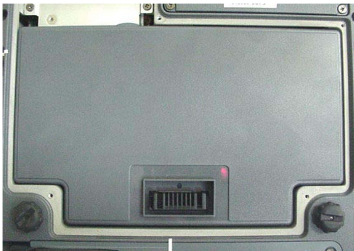
Internal Li-ion Battery 11.1 V, 3600 mAh (Model: T8M-E)
