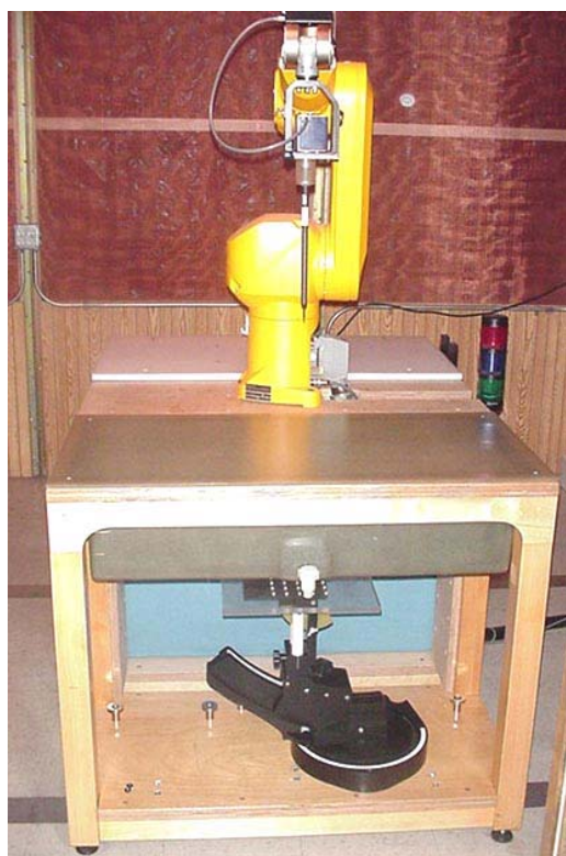
DASY4 SAR Measurement System with planar phantom
