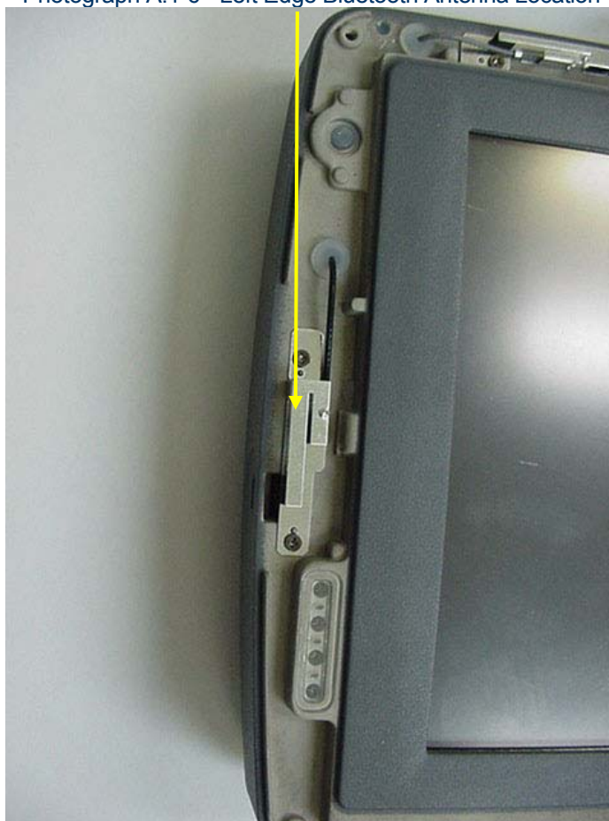
Photograph A.1-6 - Left Edge Bluetooth Antenna Location
