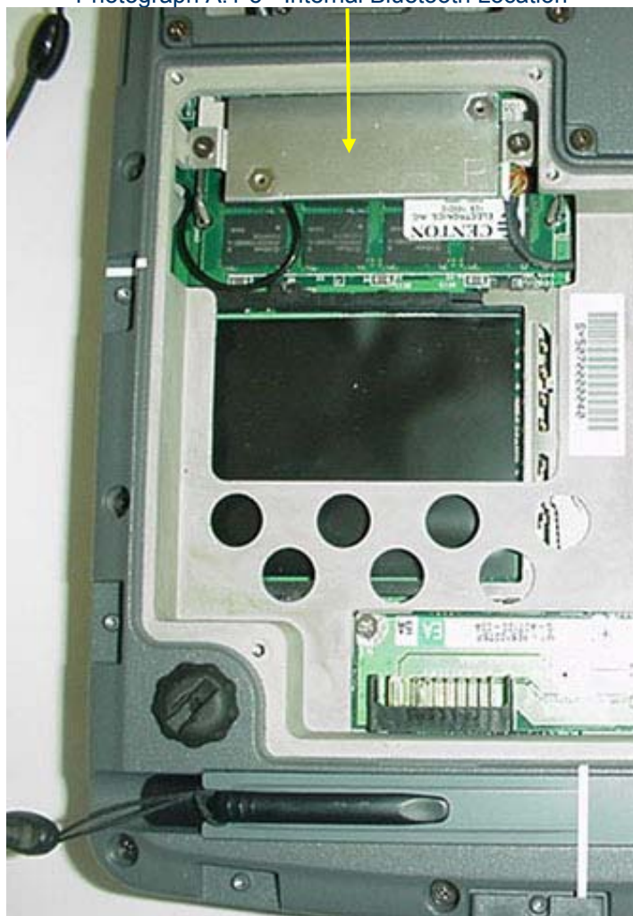
Photograph A.1-5 - Internal Bluetooth Location
