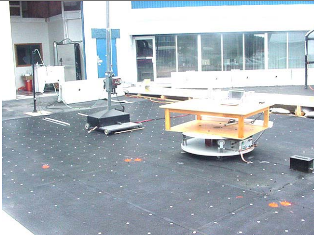
Photograph I.8-5 - 3115 Horn Antenna (10GHz - 18GHz)
