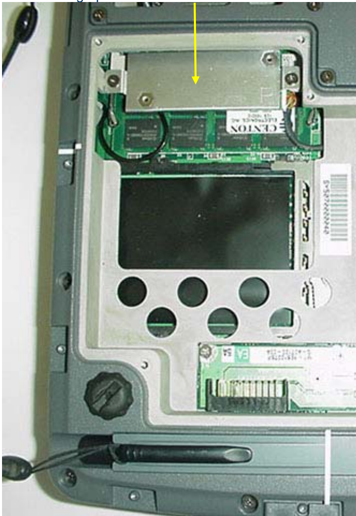
Photograph A.1-5 - Internal Bluetooth Location
