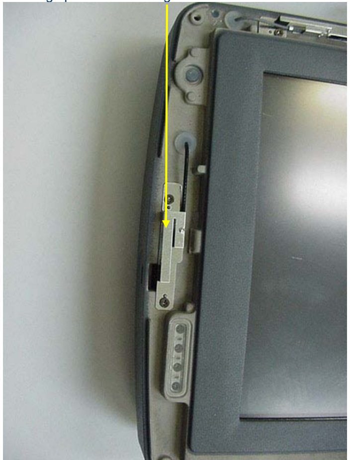
Photograph A.1-6 - Left Edge Bluetooth Antenna Location
