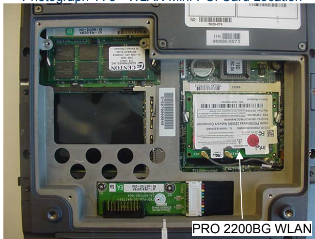
Photograph A-5 - WLAN Mini-PCI Card Location
