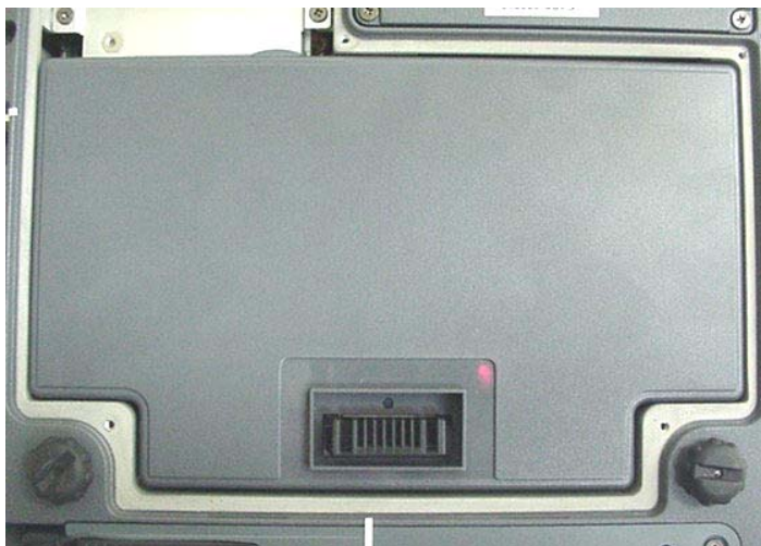
Internal Li-ion Battery 11.1 V, 3600 mAh (Model: T8M-E)
