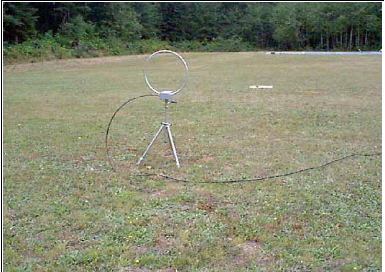
Radiated Emissions - Front View 9 kHz - 30 MHz w/antenna
