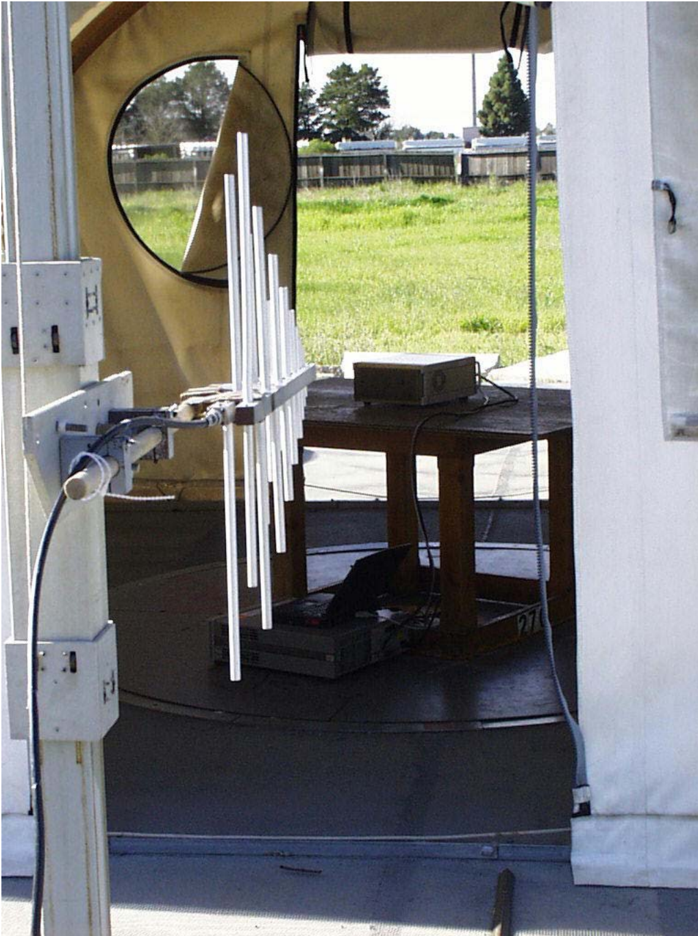
Radiated emissions test setup, LPA antenna
