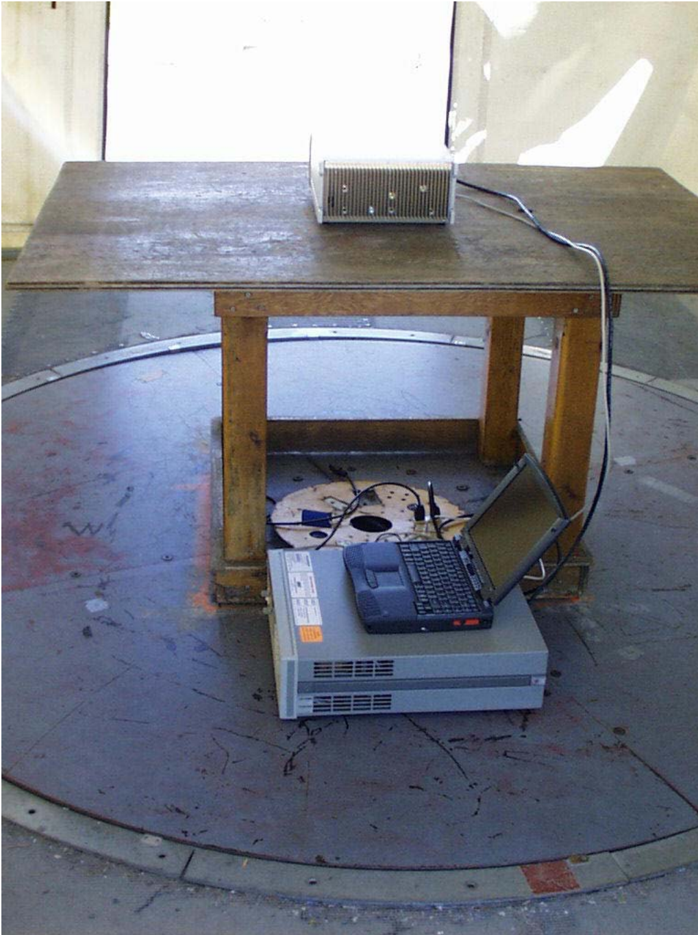
Radiated emissions, substitution method, equipment rear view
