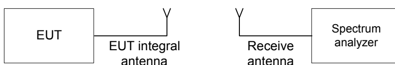
Figure 7.1.1 Setup for transmitter shut down test
