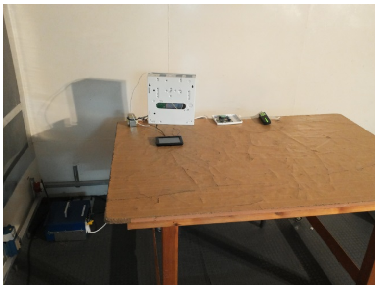
Photograph 8.1.2 Setup for conducted emission measurements
