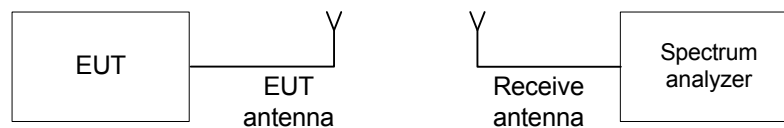
Figure 7.3.1 Occupied bandwidth test setup
