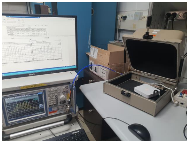
Photograph No.4 Setup for 20 dB bandwidth measurements
