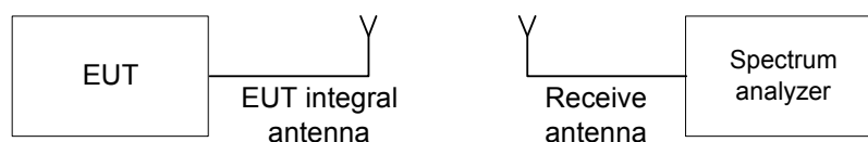
Figure 7.1.1 Setup for transmitter shut down test
