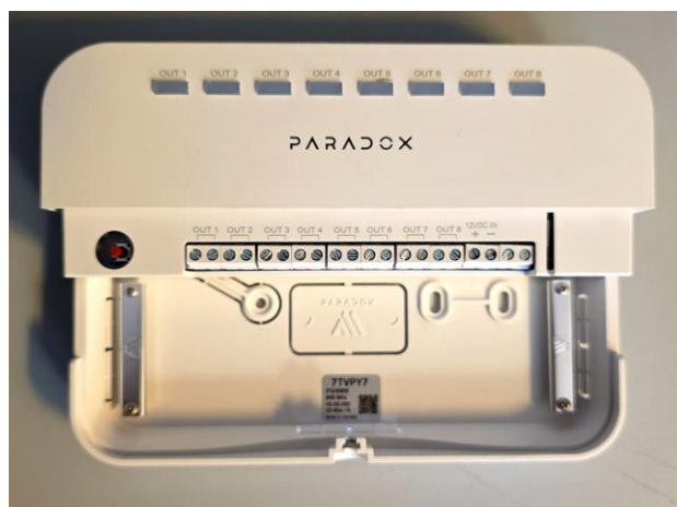
Photograph No.1 PGM8M Internal view
