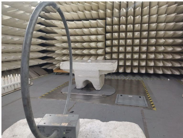
Photograph No.1 Setup for spurious field strength measurements in anechoic chamber from 9 kHz to 30 MHz
