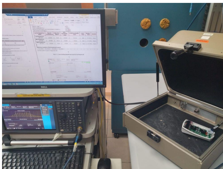
Photograph No.4 Setup for 20 dB bandwidth measurements
