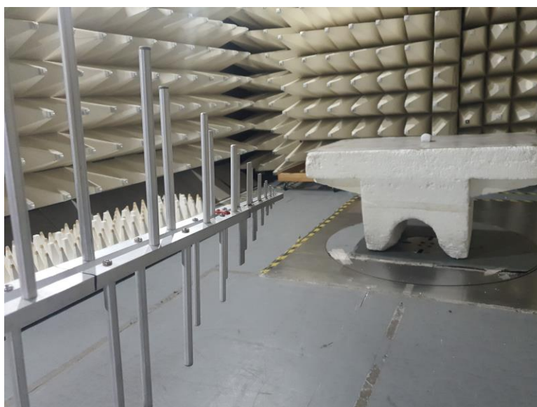
Photograph No.2 Setup for carrier and spurious emissions measurements in anechoic chamber from 30 MHz to 1 GHz
