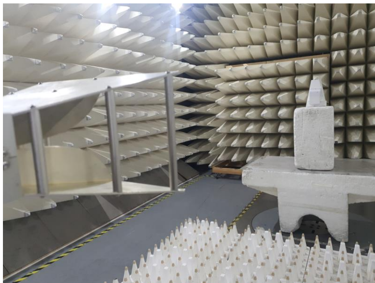
Photograph No.4 Setup for 20 dB bandwidth measurements
