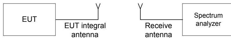
Figure 7.1.1 Setup for transmitter shut down test
