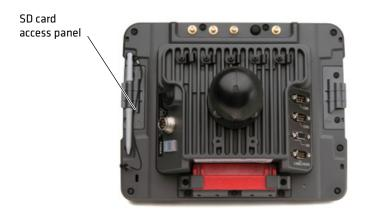
**4** Insert the SD card into the SD card slot.
