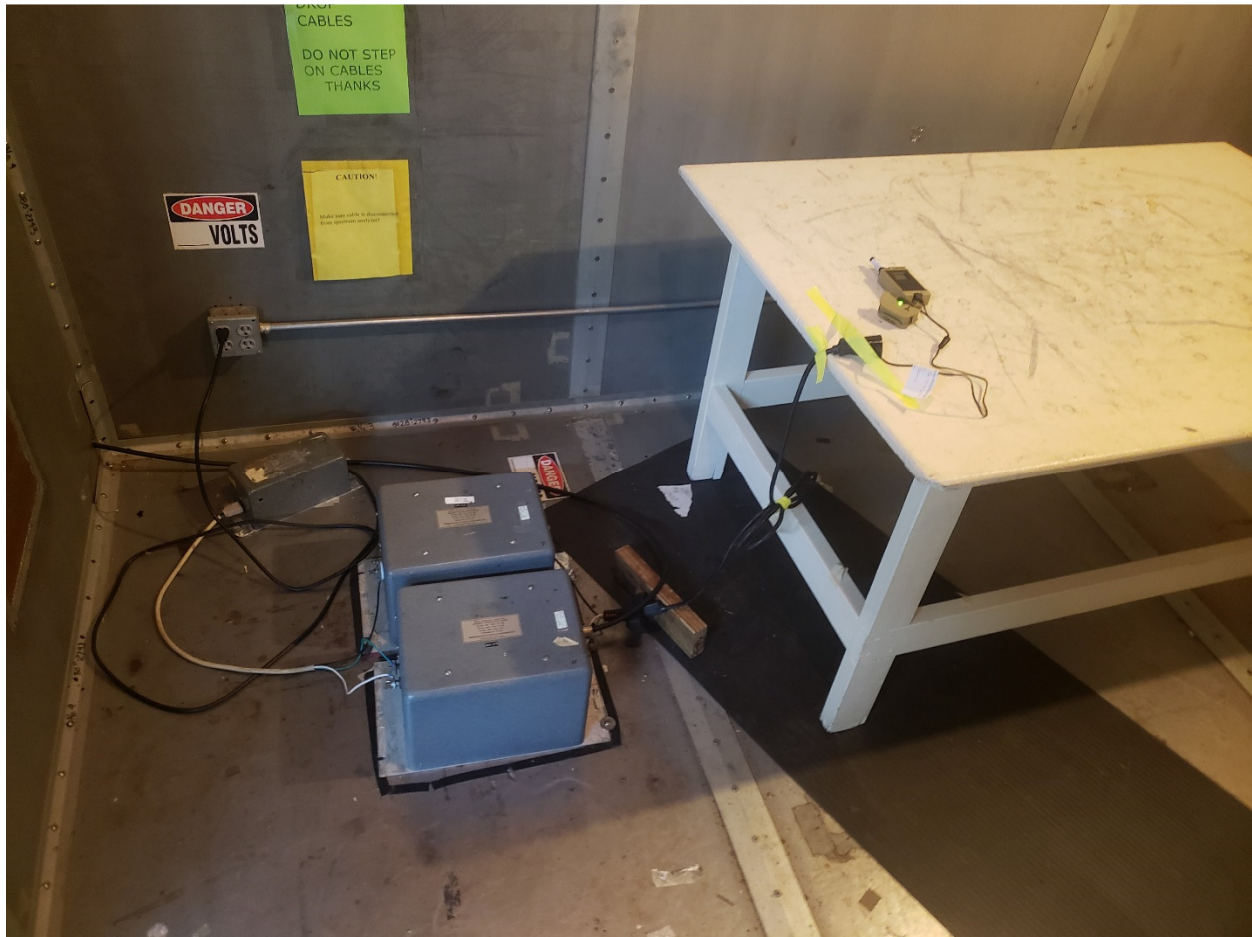
Figure 6. Power Line Conducted emissions
