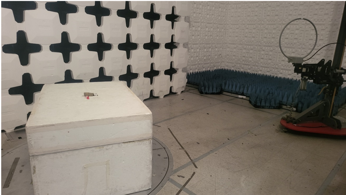
Figure 2. Radiated Emissions Test Setup, 9 kHz to 30 MHz
