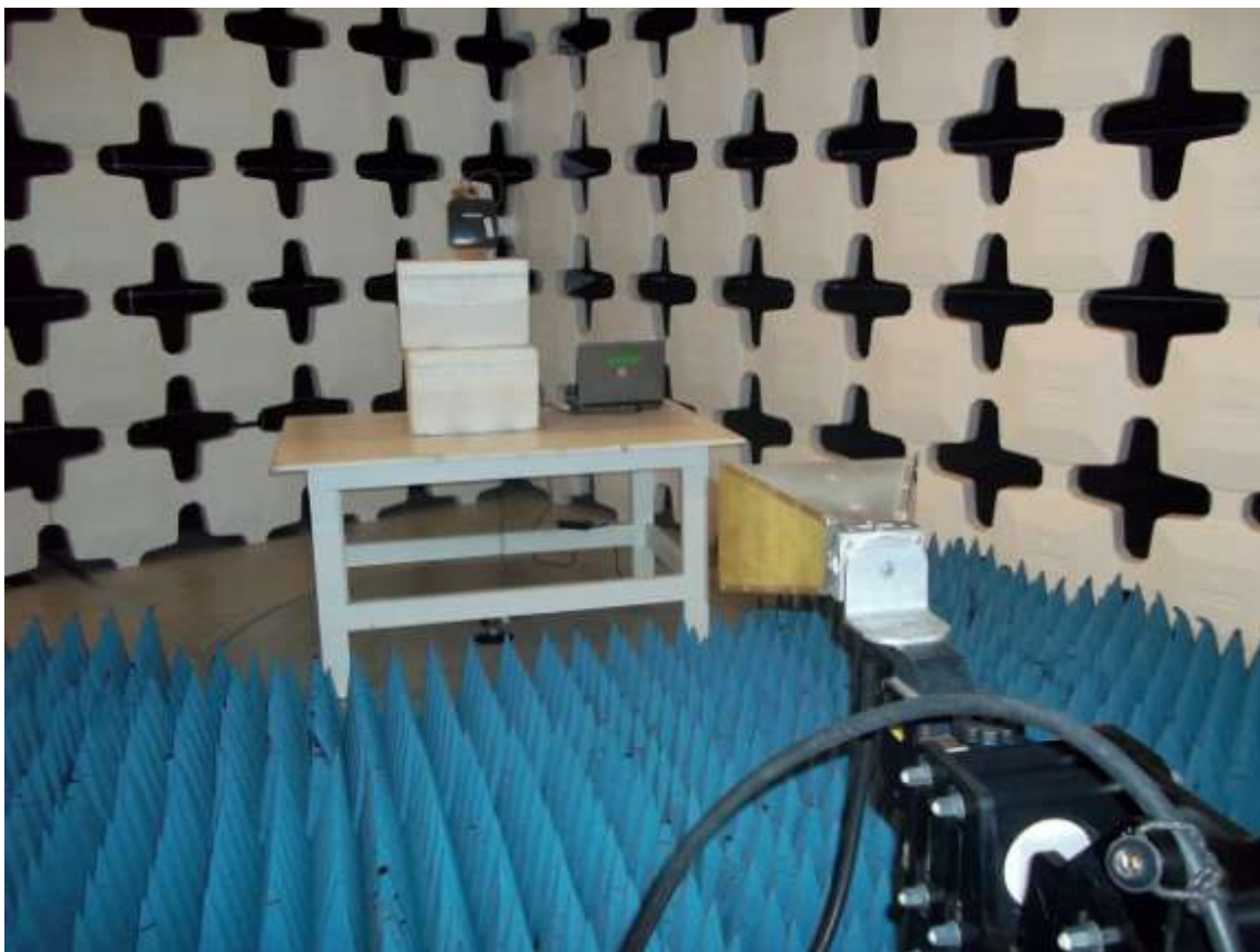
Figure 7. Radiated Emissions Test Setup, Above 1 GHz, Intentional (Radio Test with EUT in worst case position)
