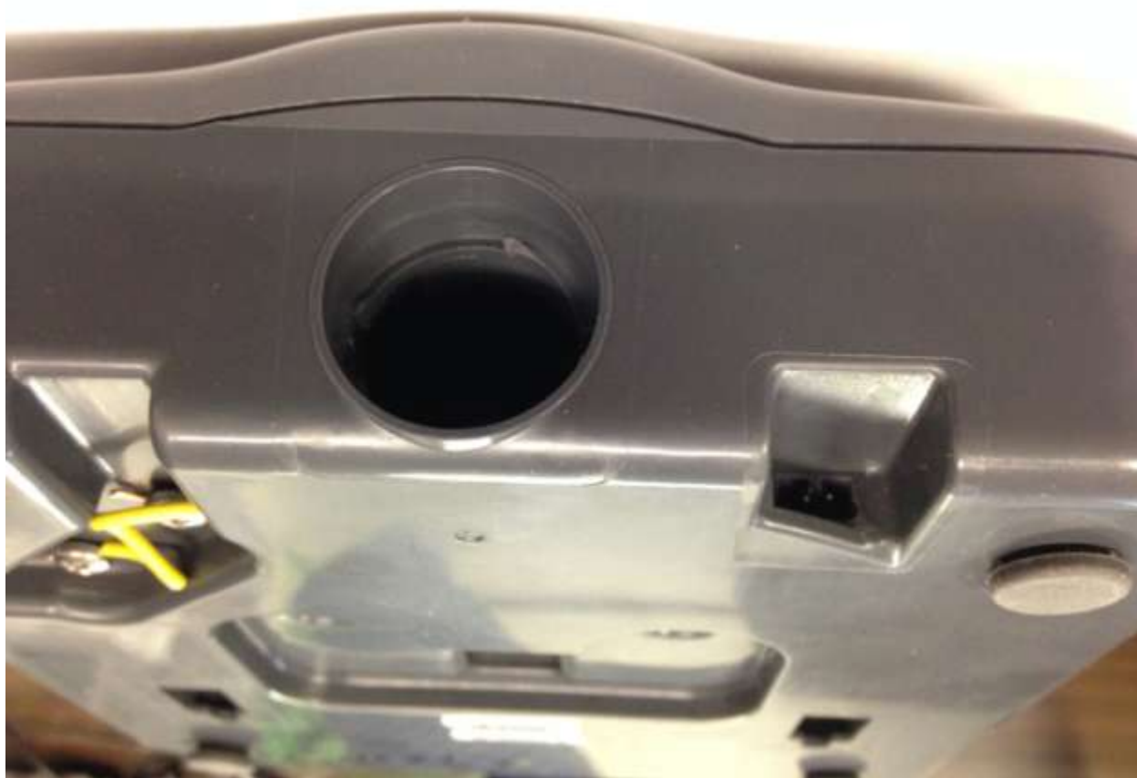
Figure 7. Battery Port and AC/DC Input Port
