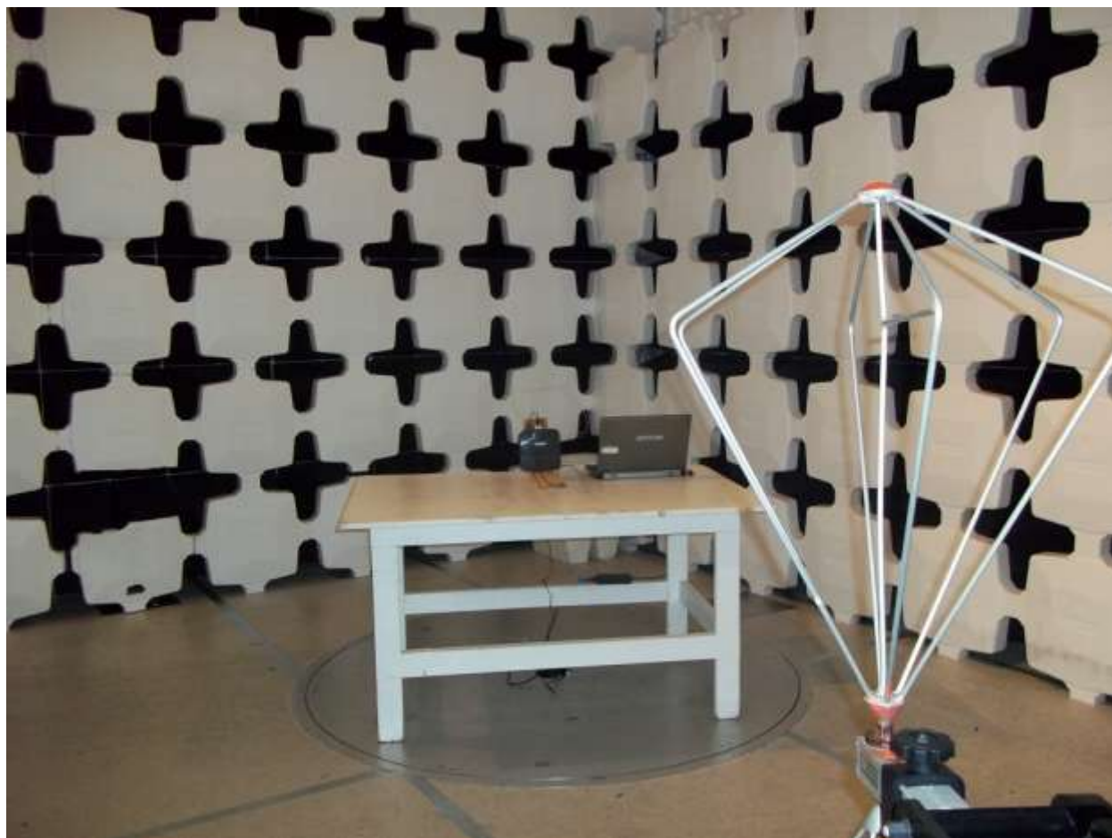
Figure 3. Radiated Emissions Test Setup (30 - 200 MHz)
