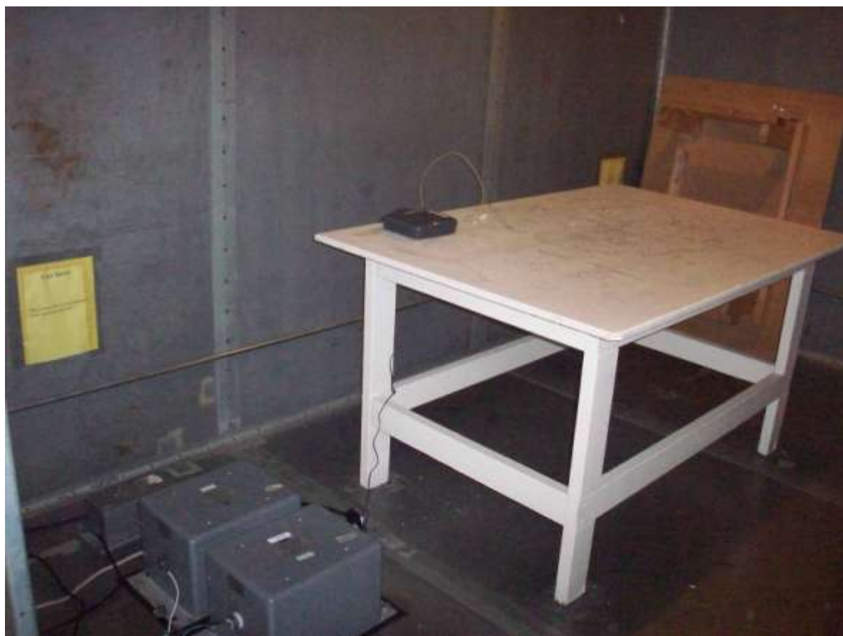
Figure 7. Power Line Conducted Emissions Test Setup
