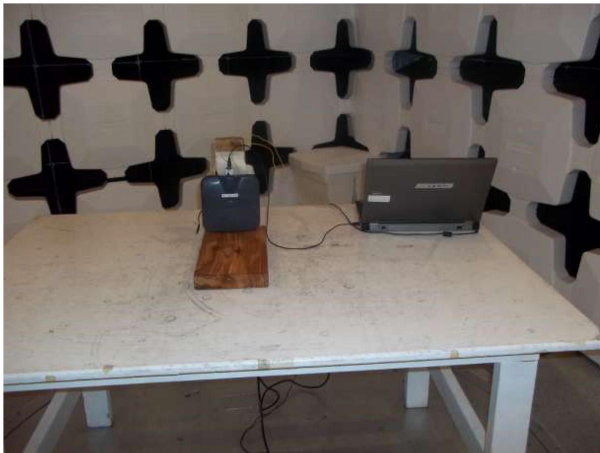
Figure 1. Radiated Emissions Test Setup, Unintentional Emissions
