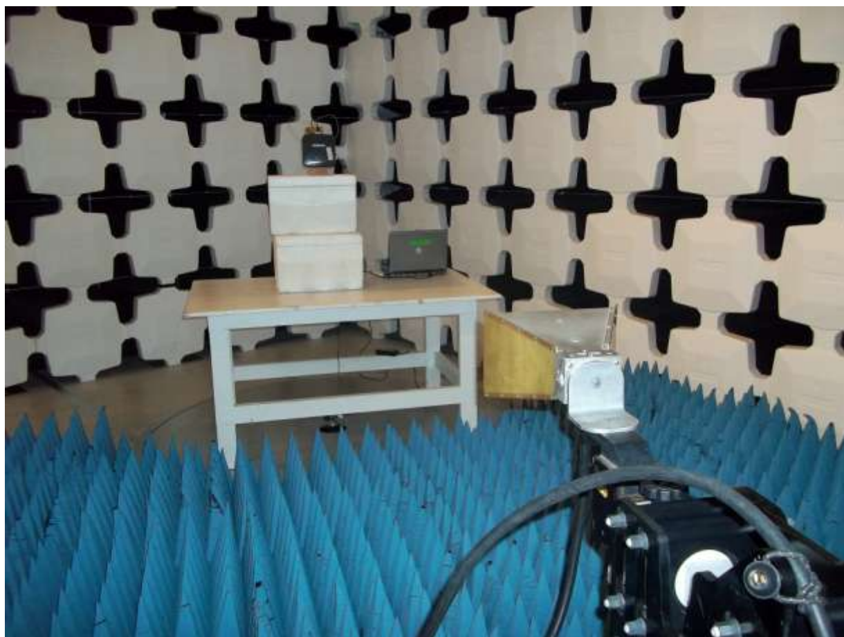
Figure 6. Radiated Emissions Test Setup (above 1 GHz – Intentional Emissions)
