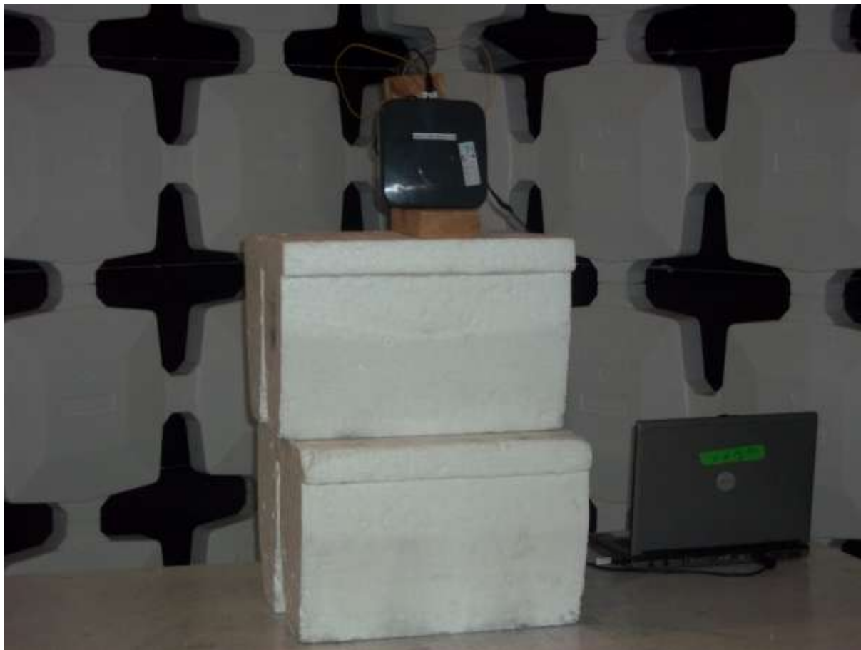
Figure 2. Radiated Emissions Test Setup, Intentional Emissions Above 1 GHz
