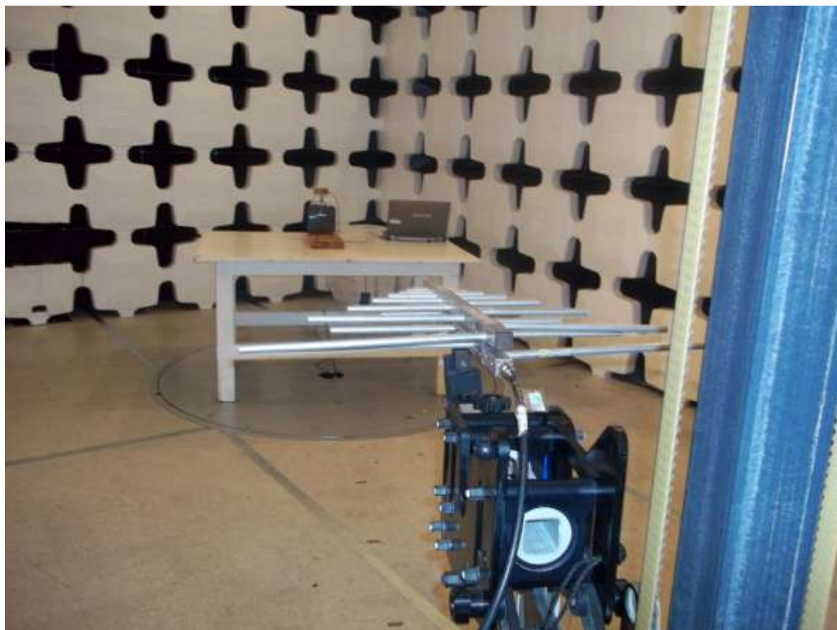
Figure 4. Radiated Emissions Test Setup (200 MHz - 1 GHz)
