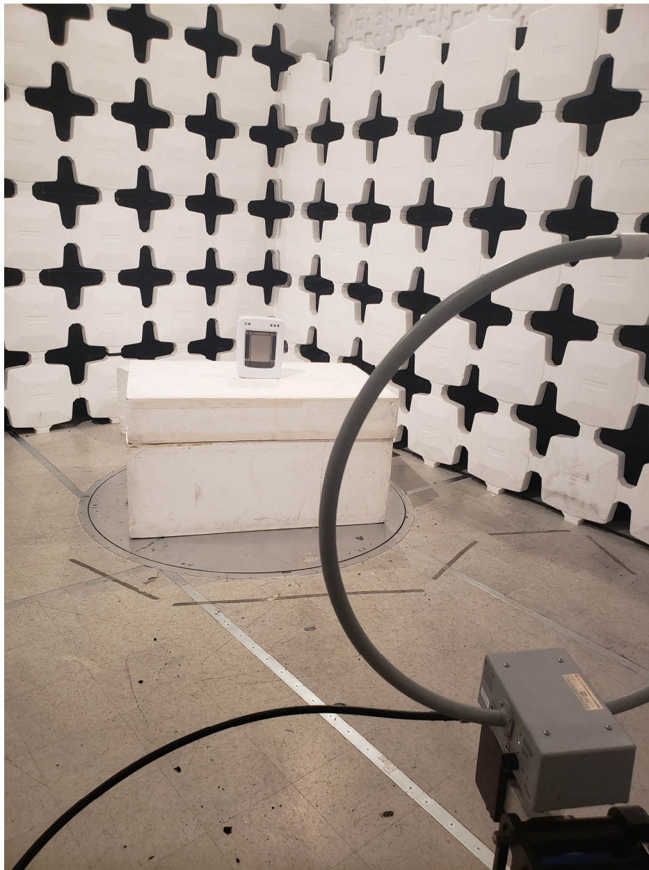
Figure 2. Radiated Emissions Test Setup, 9 kHz to 30 MHz
