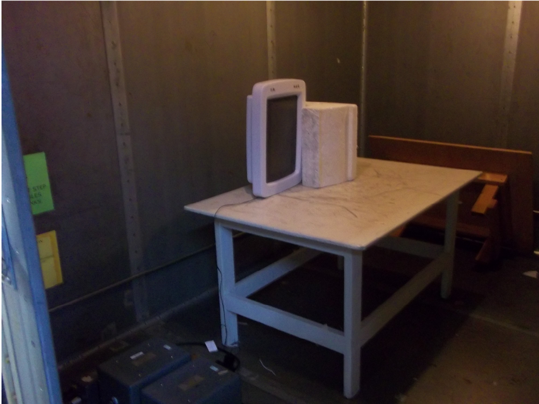
Figure 6. Powerline Conducted Emission Test Setup
