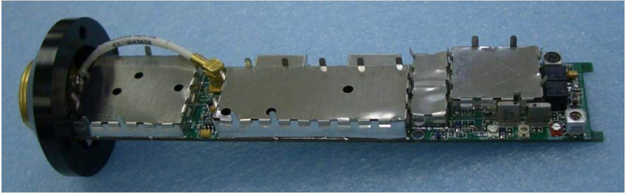
EUT – Radio PCB Top View with Shielding
