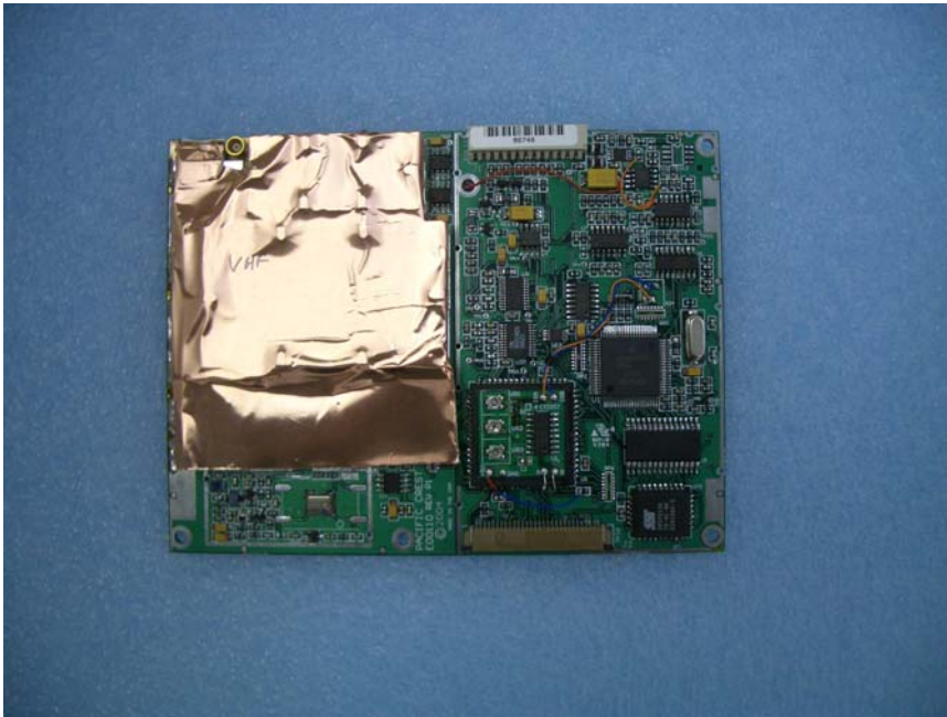
EUT – RF PCB Top View with Shielding
