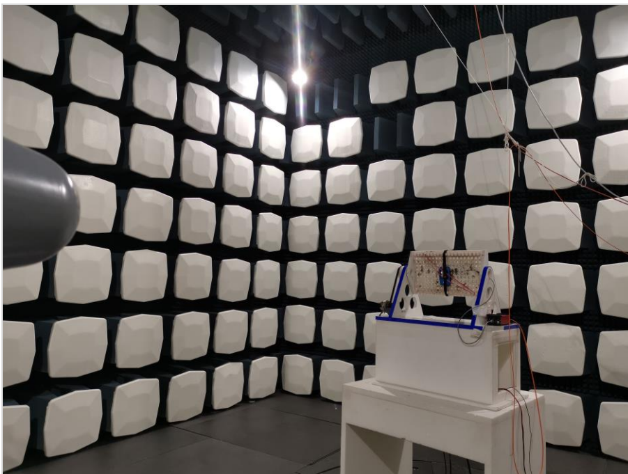
Photograph 8: EUT Test Setup in the chamber FAC1, Radiated interference field strength measured at 3 m
