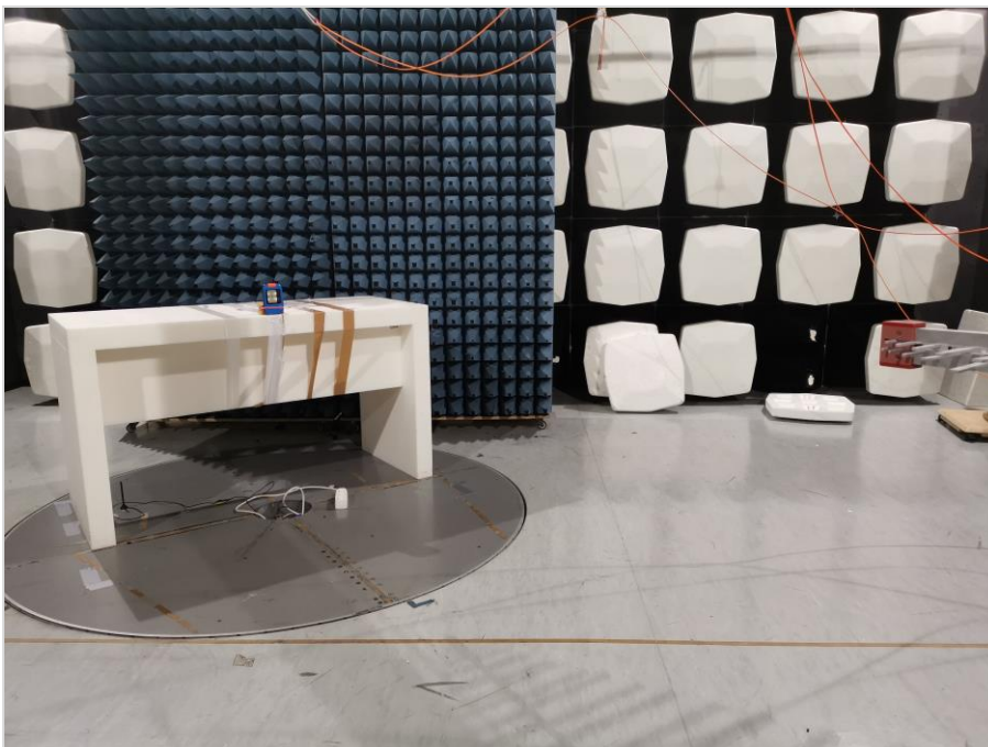
Photograph 6: EUT Test Setup in the chamber SAC1, Radiated interference field strength measured at 3 m
