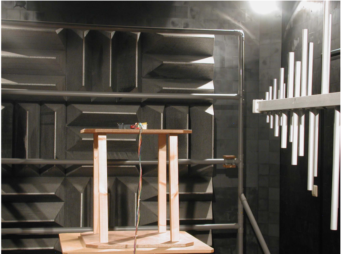
Photograph 9: Test setup radiated emissions
