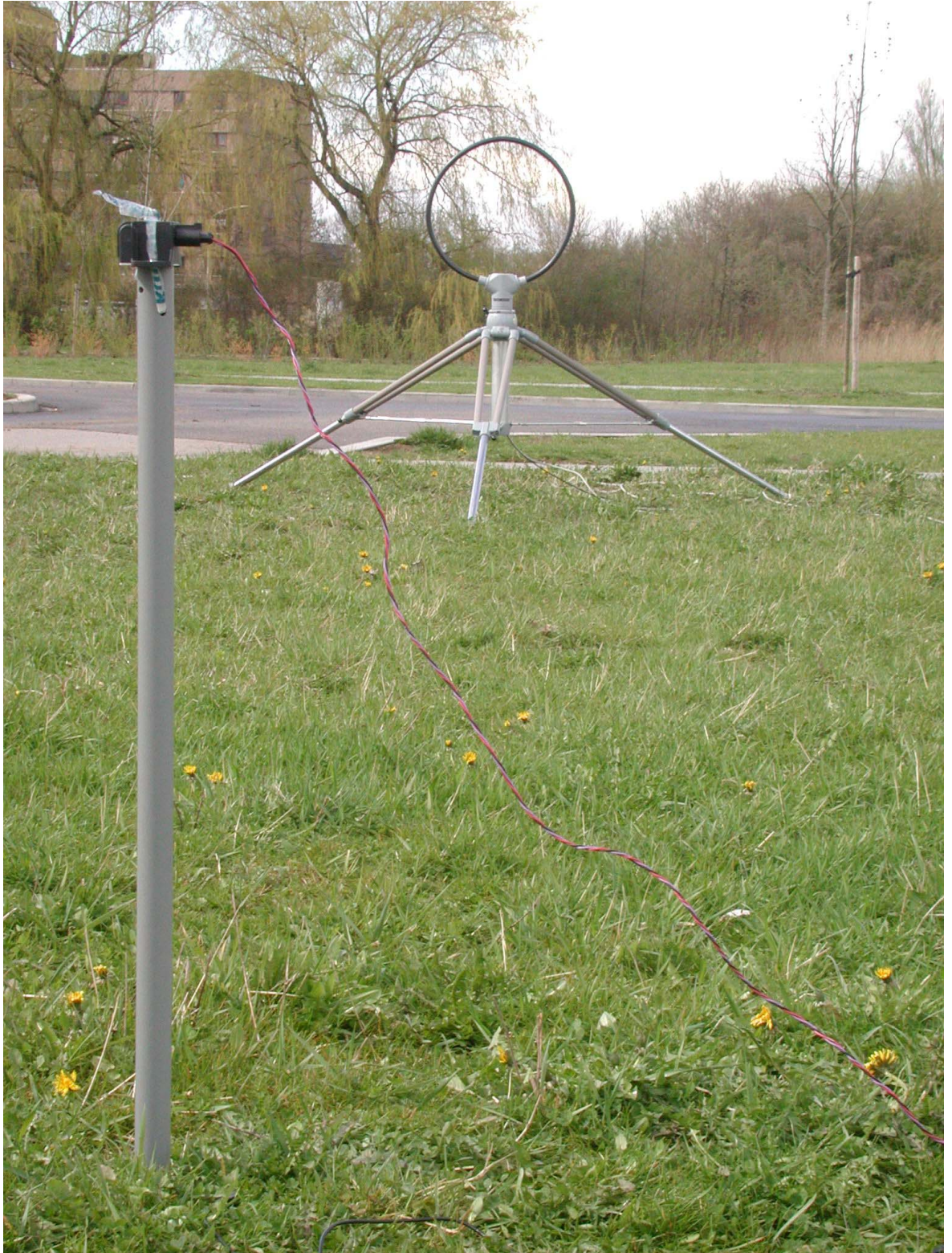
Photograph 4: 10 m test set up, ( < 30 MHz)
