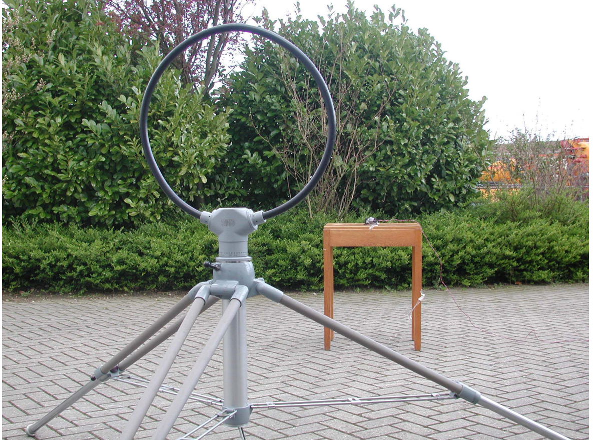
Photograph 5: 3 m test set up, ( < 30 MHz)
