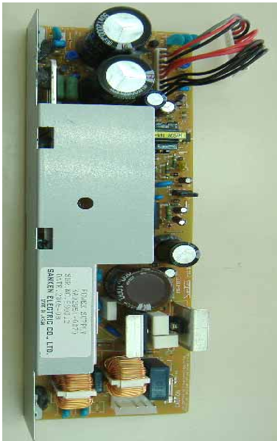
Power supply board
