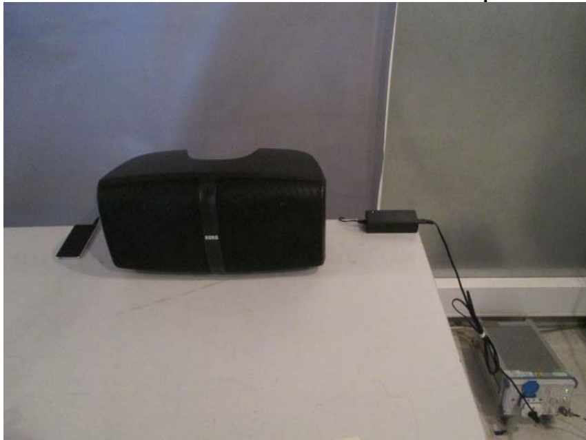
Measurement of Conducted Emission Test Set Up
