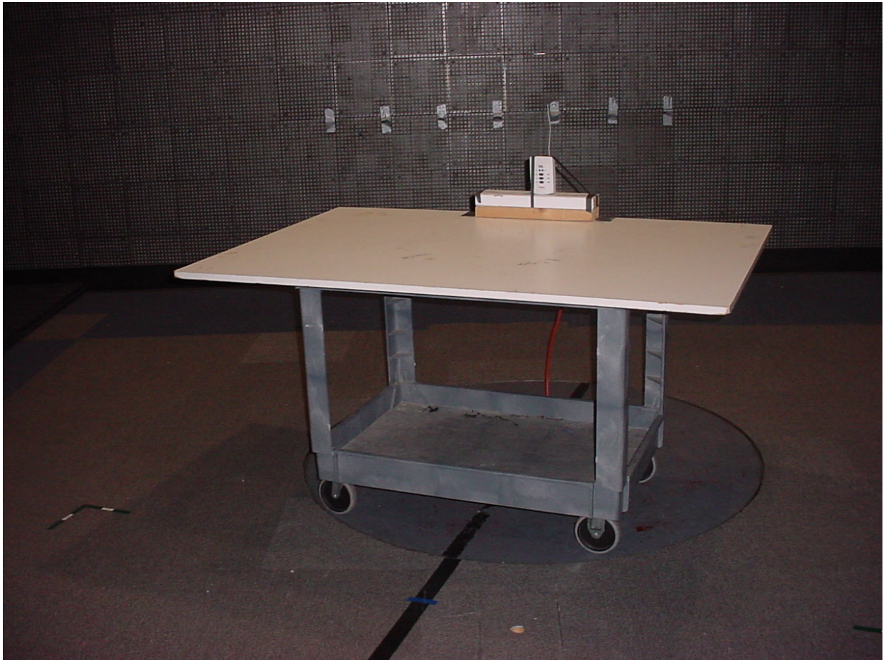
Figure 4: Test Setup – Radiated Emissions - Unintentional
