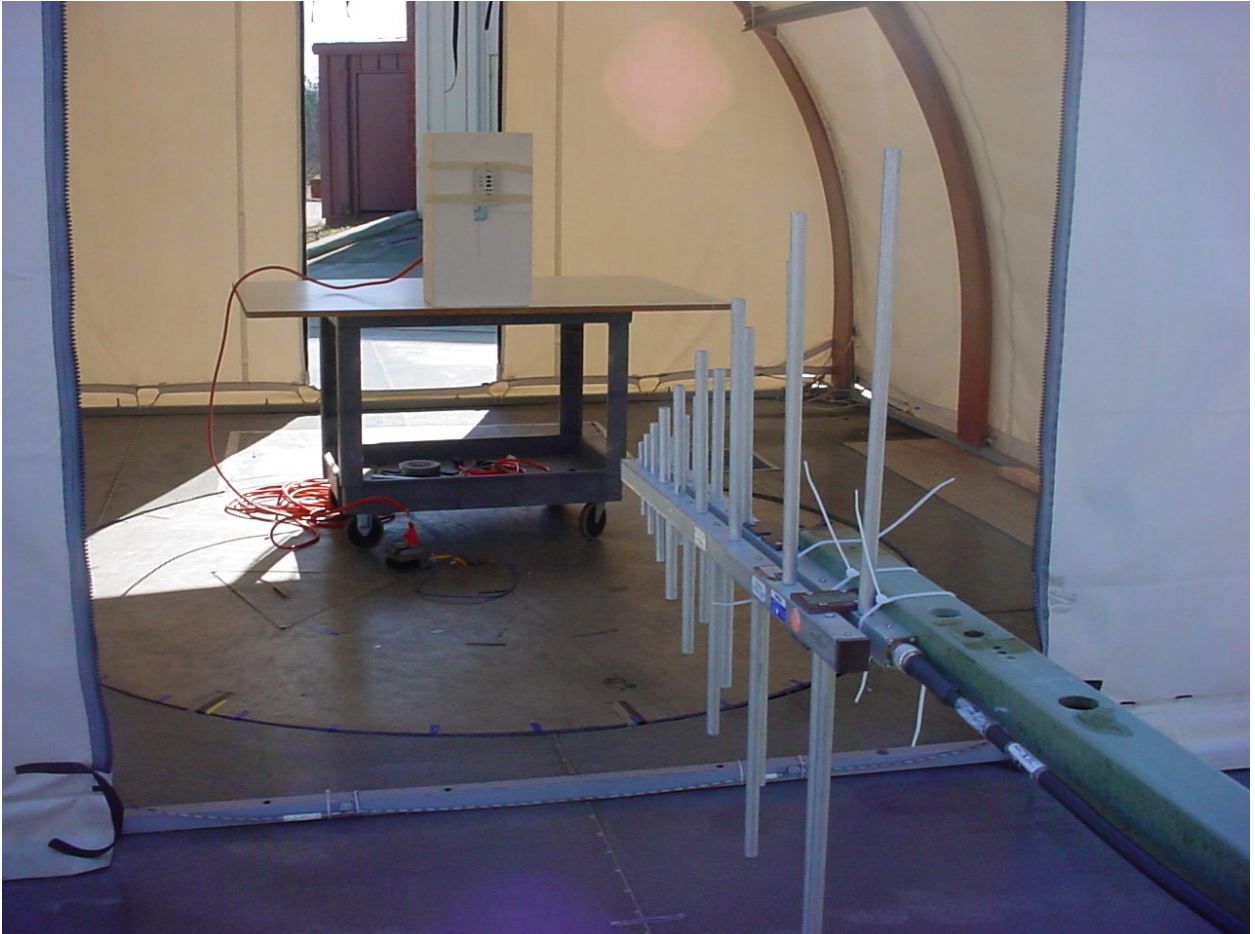
Figure 2: Test Setup – Radiated Emissions
