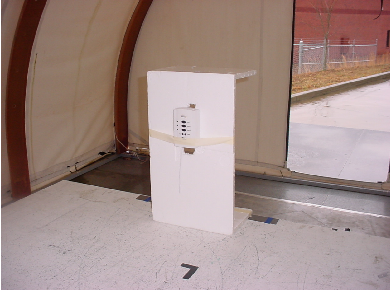
Figure 1: Test Setup – Radiated Emissions
