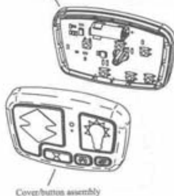
Base with circuit board and battery installed
