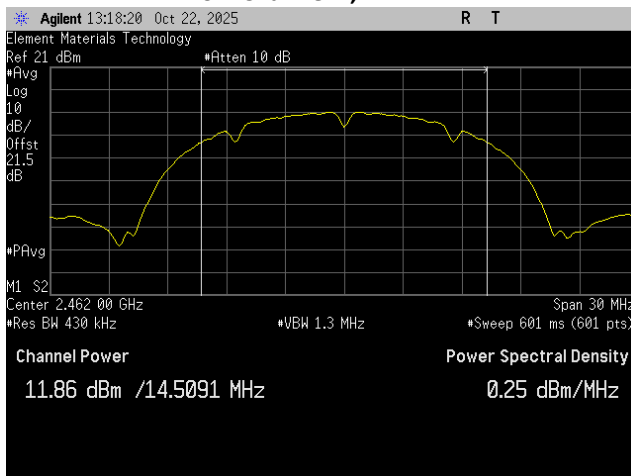
Port 1 20 MHz BW 802.11(b) 1 Mbps High Channel 11, 2462 MHz
