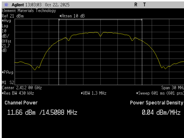
Port 1 20 MHz BW 802.11(b) 1 Mbps Low Channel 1, 2412 MHz
