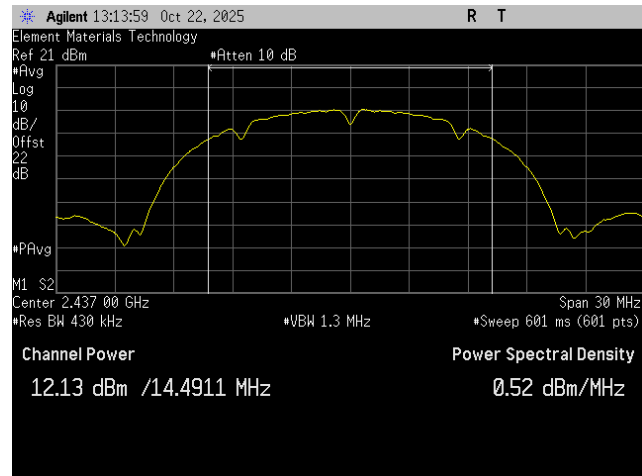
Port 1 20 MHz BW 802.11(b) 1 Mbps Mid Channel 6, 2437 MHz
