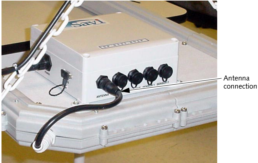
Figure 2-5 Model SP-600-201 or SP-600-211 Signpost Antenna Connection
