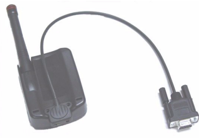
SMR-650-210 and SMR-650-213 Reader with DB-9 connector
