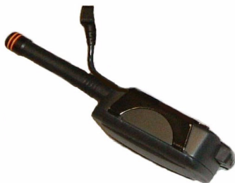
SMR-650-212 Reader with custom Intermec cable
