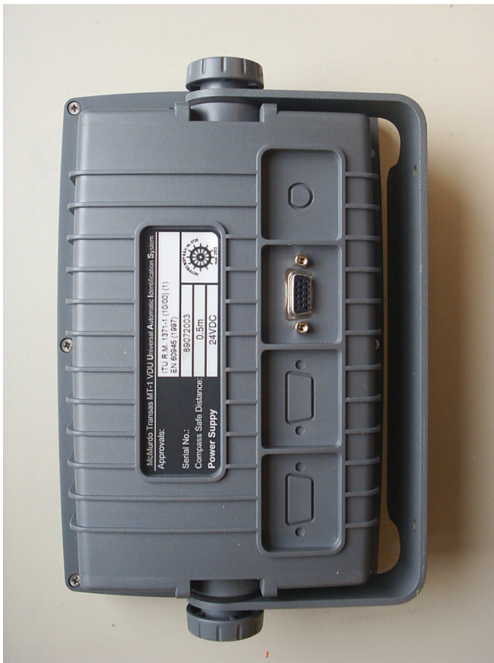
Photograph 15: Display enclosure rear side
