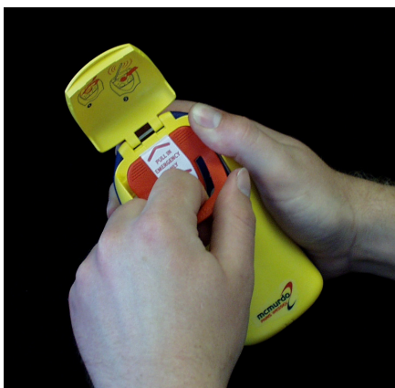
Pulling anti-tamper cover from PLB
