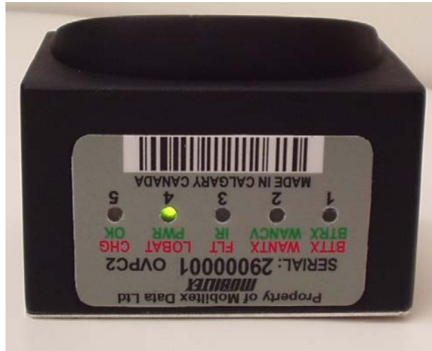
Figure 5 - OVPC Front View - LED Indicators
