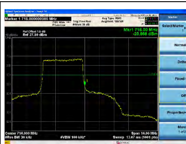
LTE Band 12, QPSK, 3MHz-High CH, 100% RB
