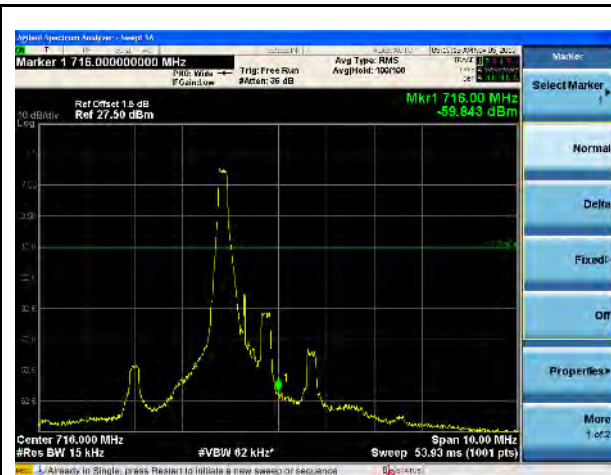
LTE Band 12, 16QAM, 1.4MHz-High CH, 1RB
