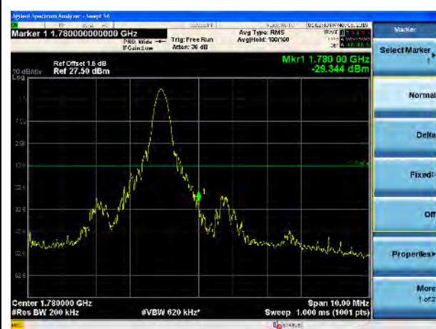
LTE Band 66, 16QAM, 20MHz-High CH, 1RB
