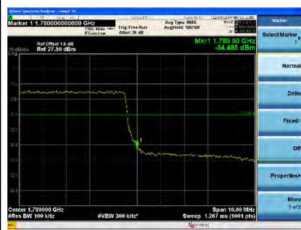
LTE Band 66, 16QAM, 10MHz-High CH, 100% RB
