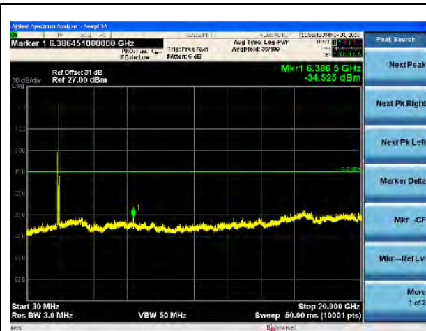
LTE Band 2, 15MHz-Mid CH
