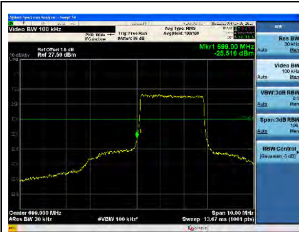
LTE Band 12, 16QAM, 3MHz-Low CH, 100% RB
