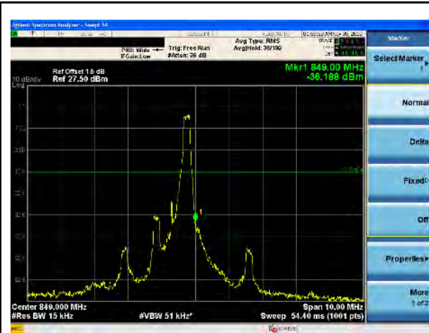
LTE Band 5, QPSK, 1.4MHz-High CH, 1RB
