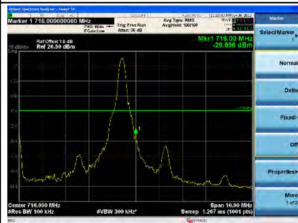
LTE Band 17, QPSK, 10MHz-High CH, 1RB
