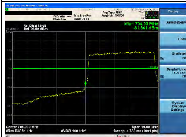
LTE Band 17, 16QAM, 5MHz-Low CH, 100% RB
