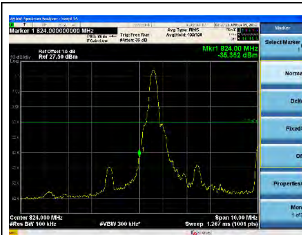
LTE Band 5, QPSK, 10MHz-Low CH, 1RB
