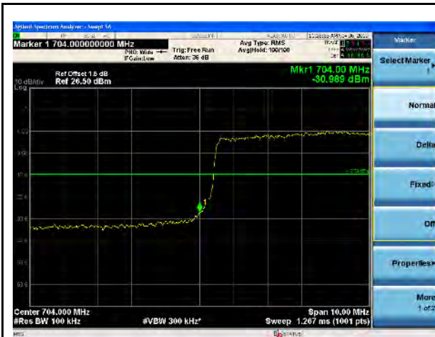
LTE Band 17, QPSK, 10MHz-Low CH, 100% RB
