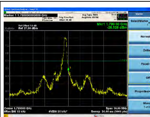
LTE Band 66, 16QAM, 1.4MHz-High CH, 1RB
