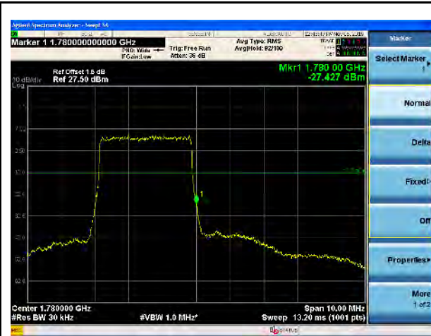
LTE Band 66, QPSK, 3MHz-High CH, 100% RB
