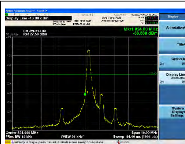
LTE Band 5, QPSK, 1.4MHz-Low CH, 1RB
