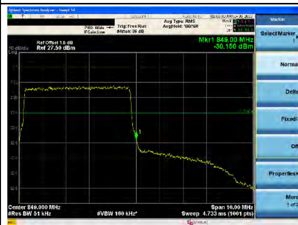
LTE Band 5, QPSK, 5MHz-High CH, 100% RB
