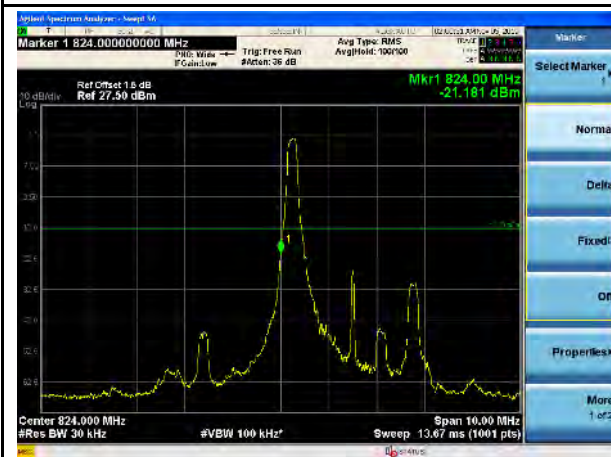
LTE Band 5, QPSK, 3MHz-Low CH, 1RB
