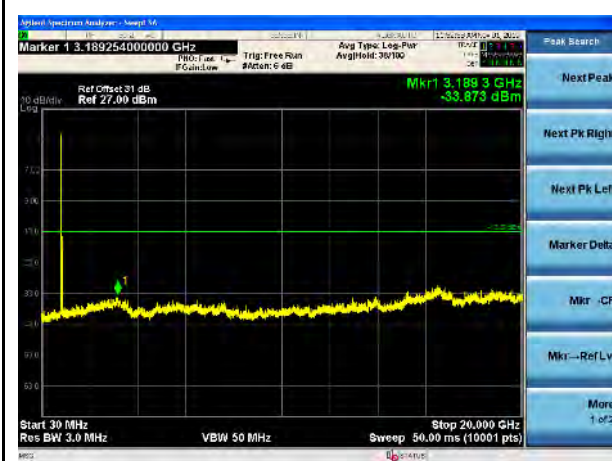
LTE Band 5, 5MHz-High CH
