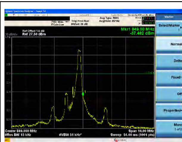
LTE Band 5, 16QAM, 1.4MHz-High CH, 1RB
