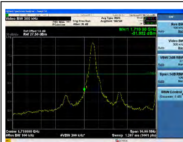
LTE Band 66, 16QAM, 10MHz-Low CH, 1RB
