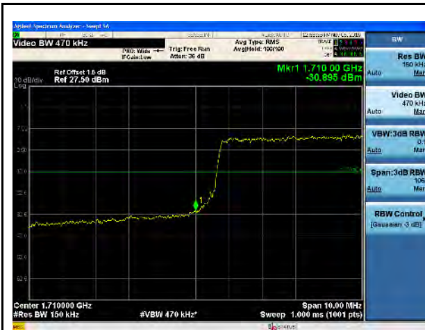
LTE Band 66, QPSK, 15MHz-Low CH, 100% RB
