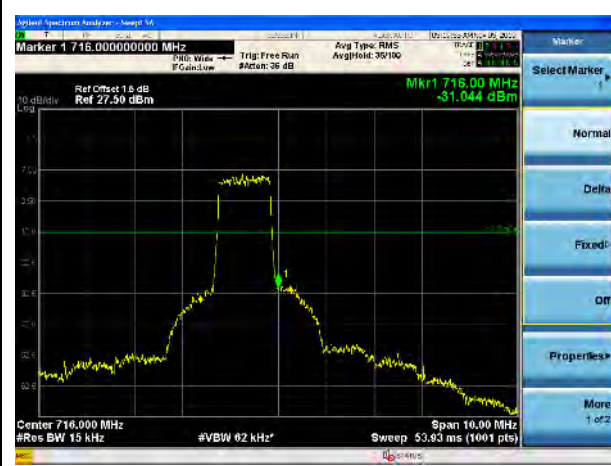
LTE Band 12, QPSK, 1.4MHz-High CH, 100% RB
