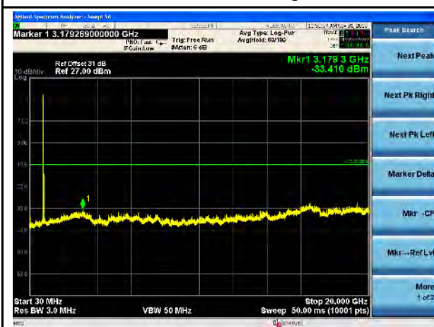
LTE Band 5, 3MHz-Mid CH
