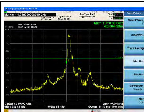
LTE Band 66, 16QAM, 1.4MHz-Low CH, 1RB
