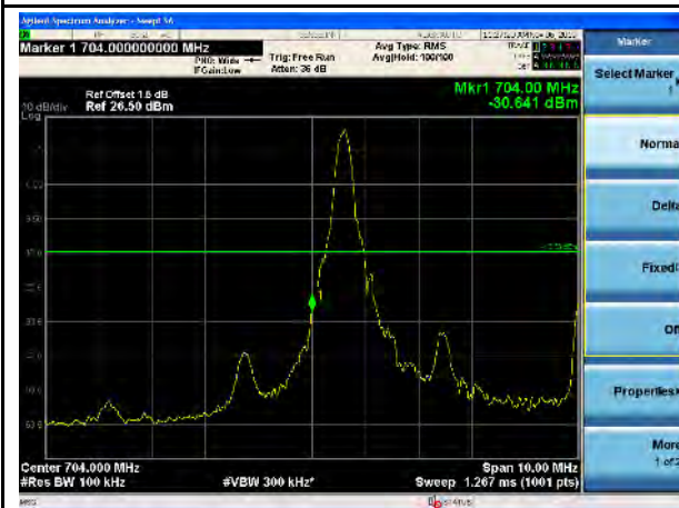
LTE Band 17, QPSK, 10MHz-Low CH, 1RB
