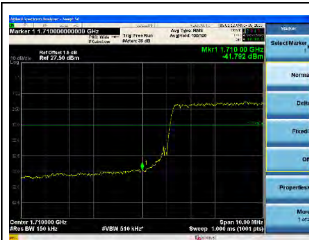
LTE Band 4, 16QAM, 15MHz-Low CH, 100% RB
