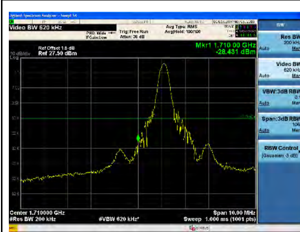
LTE Band 66, QPSK, 20MHz-Low CH, 1RB
