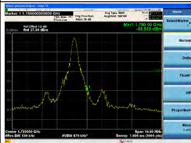
LTE Band 66, 16QAM, 15MHz-High CH, 1RB
