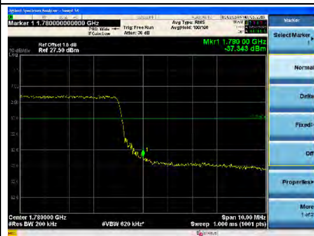
LTE Band 66, 16QAM, 20MHz-High CH, 100% RB
