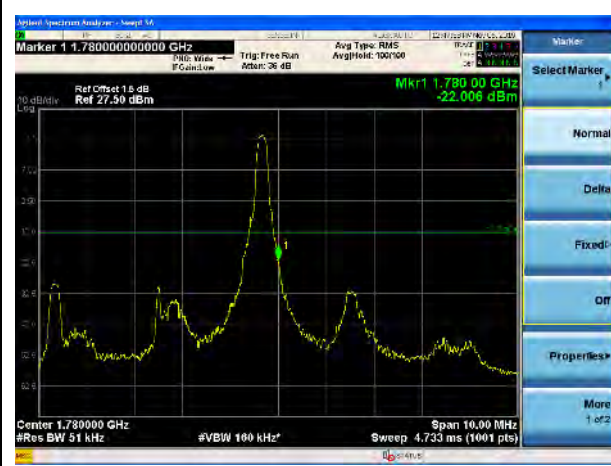
LTE Band 66, QPSK, 5MHz-High CH, 1RB
