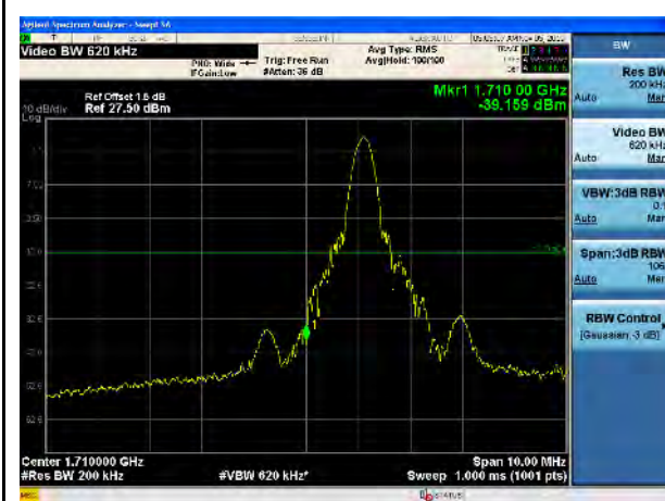
LTE Band 4, 16QAM, 20MHz-Low CH, 1RB
