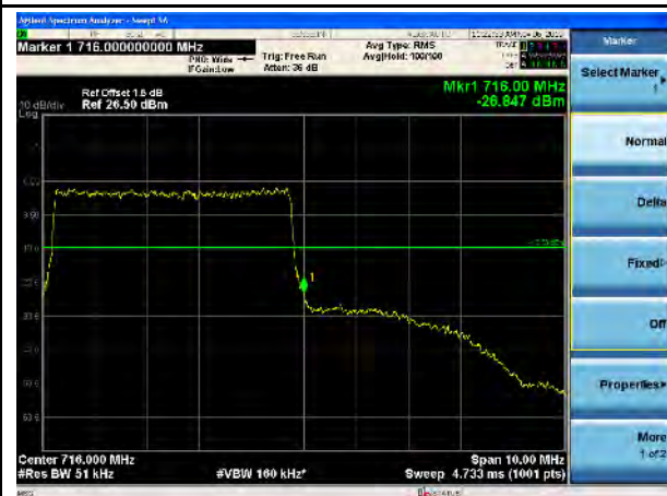
LTE Band 17, 16QAM, 5MHz-High CH, 100% RB
