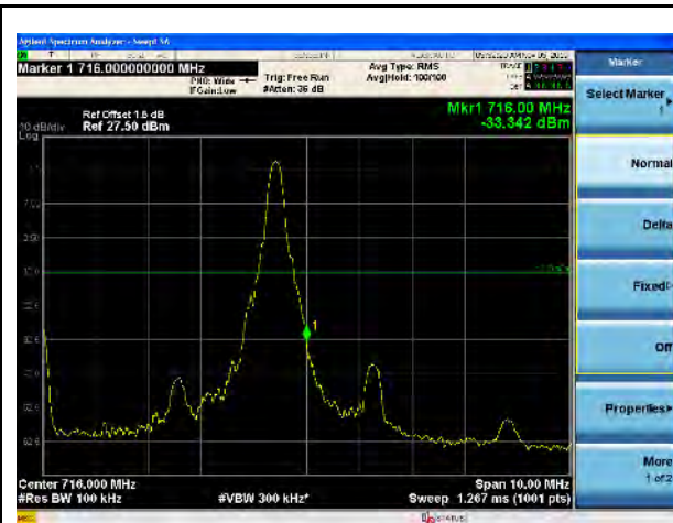
LTE Band 12, 16QAM, 10MHz-High CH, 1RB
