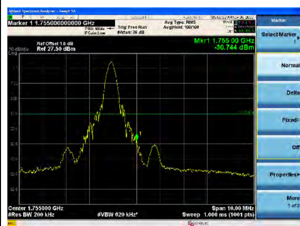
LTE Band 4, 16QAM, 20MHz-High CH, 1RB
