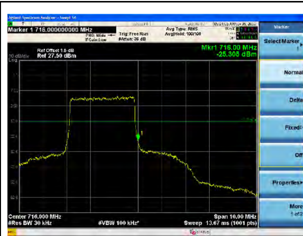
LTE Band 12, 16QAM, 3MHz-High CH, 100% RB
