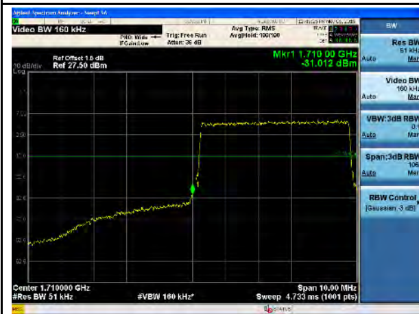
LTE Band 66, 16QAM, 5MHz-Low CH, 100% RB
