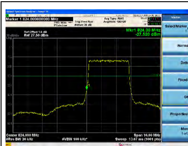
LTE Band 5, QPSK, 3MHz-Low CH, 100% RB
