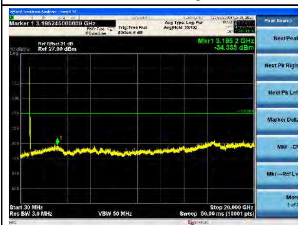
LTE Band 5, 10MHz-Mid CH
