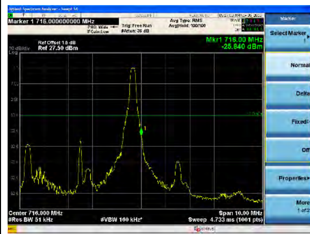
LTE Band 12, 16QAM, 5MHz-High CH, 1RB
