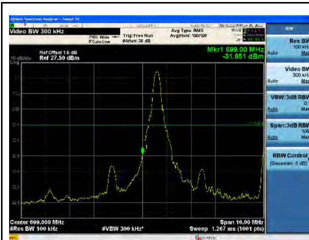
LTE Band 12, QPSK, 10MHz-Low CH, 1RB
