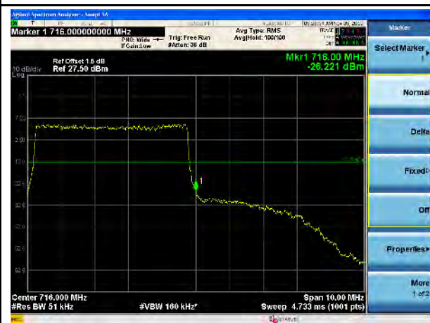
LTE Band 12, QPSK, 5MHz-High CH, 100% RB
