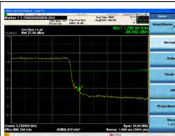
LTE Band 66, 16QAM, 15MHz-High CH, 100% RB
