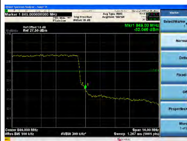
LTE Band 5, QPSK, 10MHz-High CH, 100% RB
