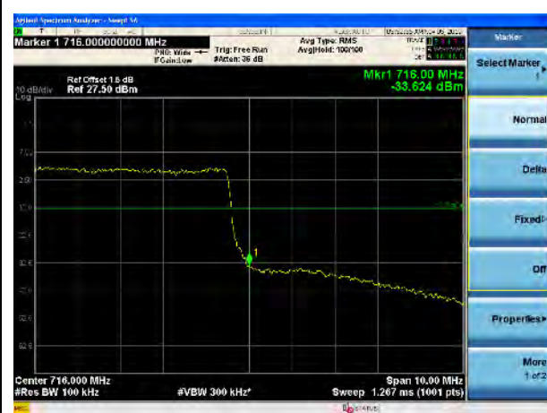
LTE Band 12, 16QAM, 10MHz-High CH, 100% RB
