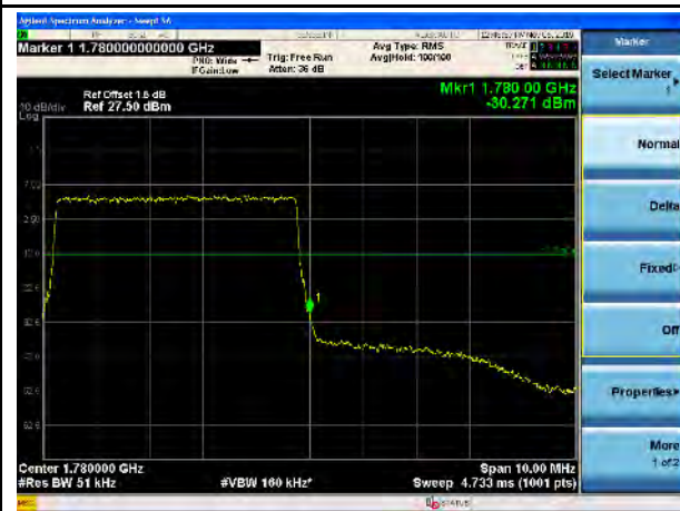
LTE Band 66, QPSK, 5MHz-High CH, 100% RB
