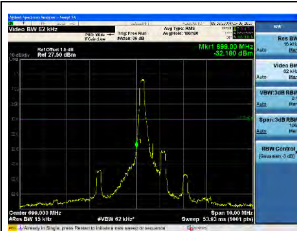
LTE Band 12, QPSK, 1.4MHz-Low CH, 1RB
