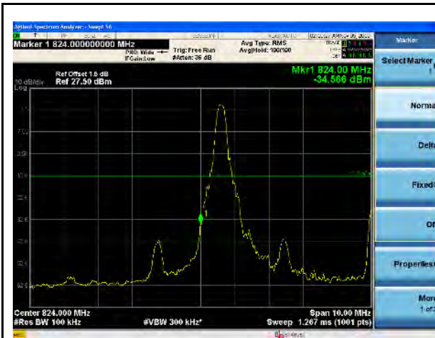
LTE Band 5, 16QAM, 10MHz-Low CH, 1RB
