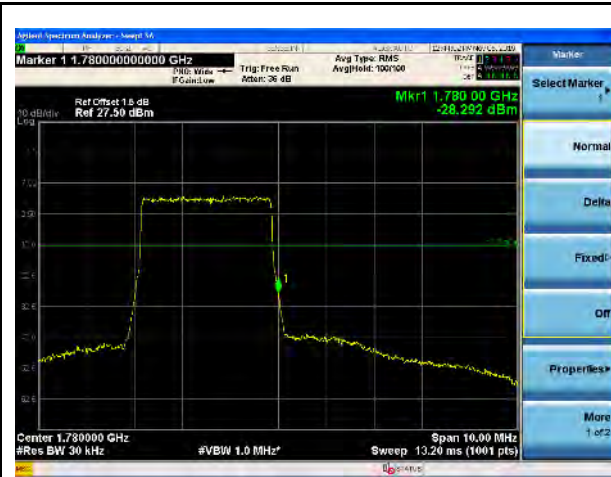
LTE Band 66, 16QAM, 3MHz-High CH, 100% RB
