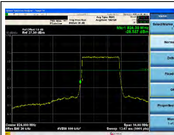
LTE Band 5, 16QAM, 3MHz-Low CH, 100% RB
