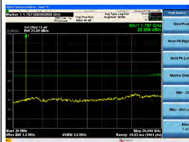
LTE Band 66, 1.4MHz-High CH
