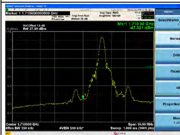
LTE Band 4, 16QAM, 15MHz-Low CH, 1RB
