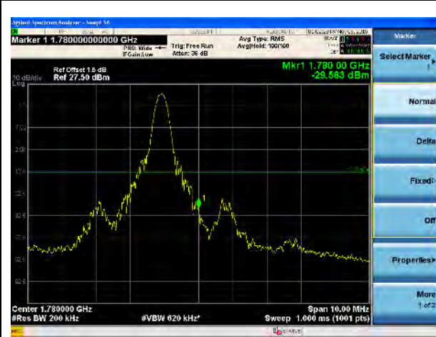
LTE Band 66, QPSK, 20MHz-High CH, 1RB
