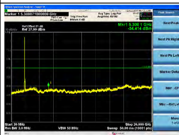
LTE Band 2, 20MHz-High CH
