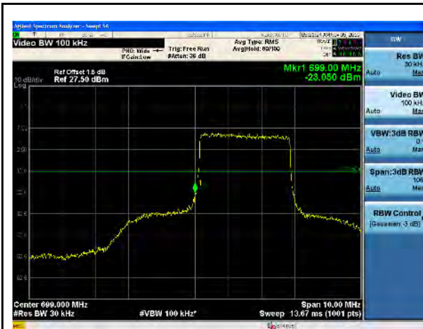
LTE Band 12, QPSK, 3MHz-Low CH, 100% RB
