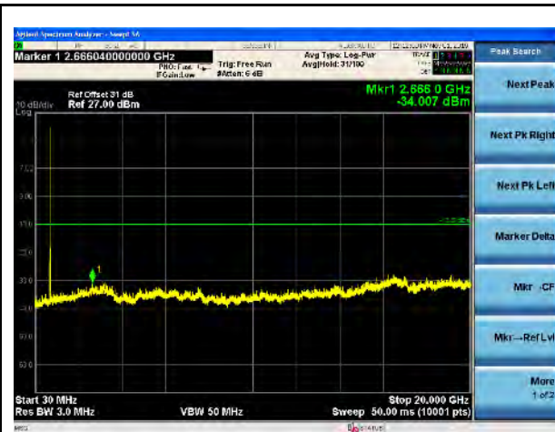
LTE Band 12, 1.4MHz-Mid CH
