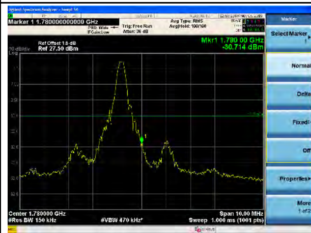
LTE Band 66, QPSK, 15MHz-High CH, 1RB
