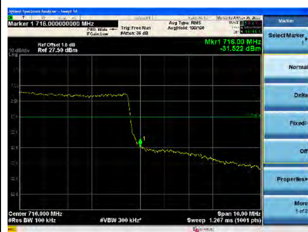
LTE Band 12, QPSK, 10MHz-High CH, 100% RB
