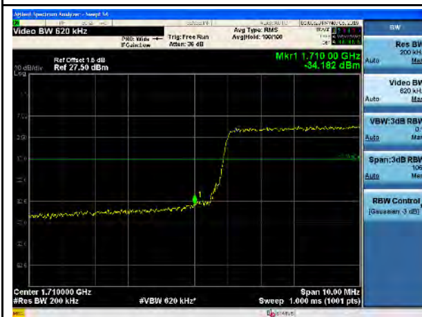
LTE Band 66, 16QAM, 20MHz-Low CH, 100% RB
