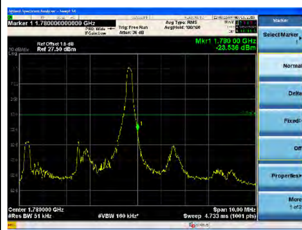
LTE Band 66, 16QAM, 5MHz-High CH, 1RB
