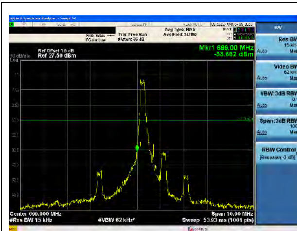
LTE Band 12, 16QAM, 1.4MHz-Low CH, 1RB
