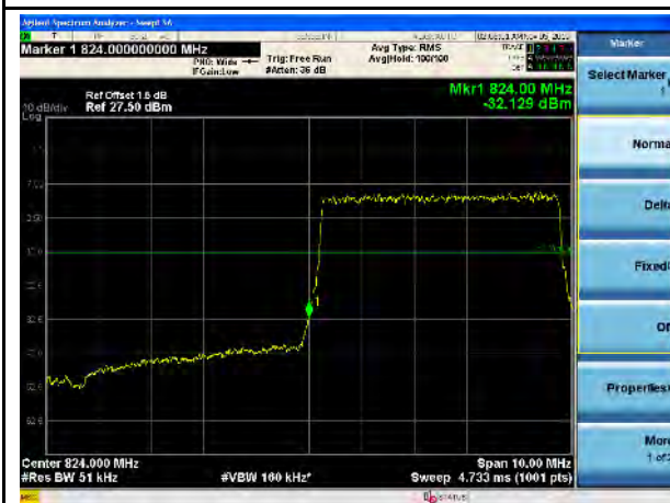
LTE Band 5, QPSK, 5MHz-Low CH, 100% RB
