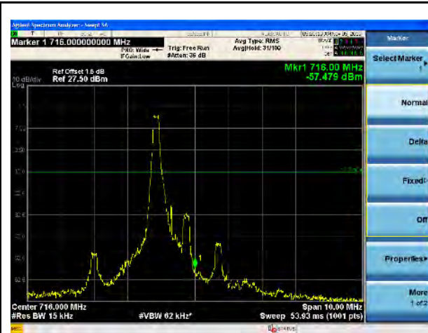
LTE Band 12, QPSK, 1.4MHz-High CH, 1RB
