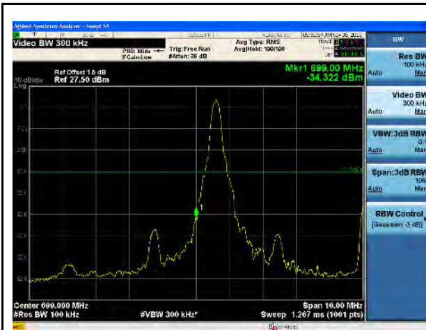
LTE Band 12, 16QAM, 10MHz-Low CH, 1RB
