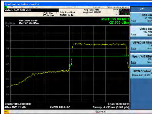
LTE Band 12, 16QAM, 5MHz-Low CH, 100% RB
