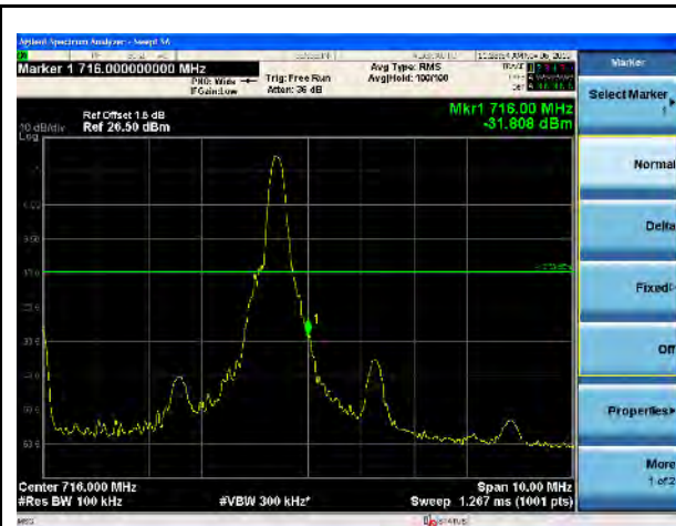
LTE Band 17, 16QAM, 10MHz-High CH, 1RB
