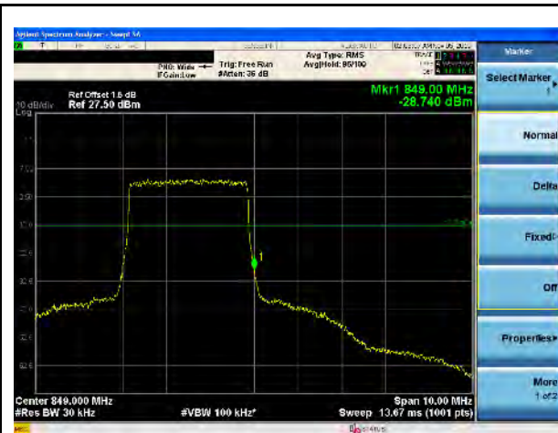
LTE Band 5, 16QAM, 3MHz-High CH, 100% RB
