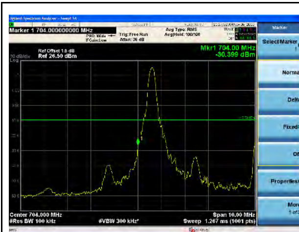
LTE Band 17, 16QAM, 10MHz-Low CH, 1RB
