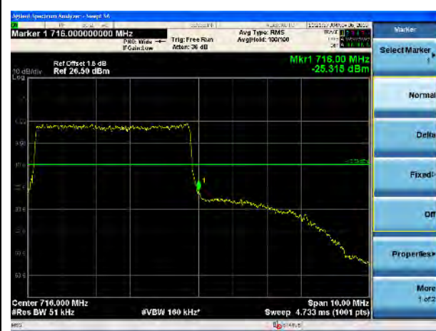
LTE Band 17, QPSK, 5MHz-High CH, 100% RB
