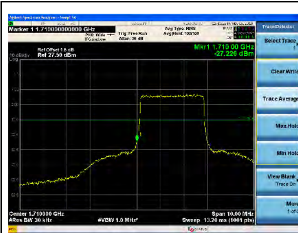
LTE Band 66, 16QAM, 3MHz-Low CH, 100% RB
