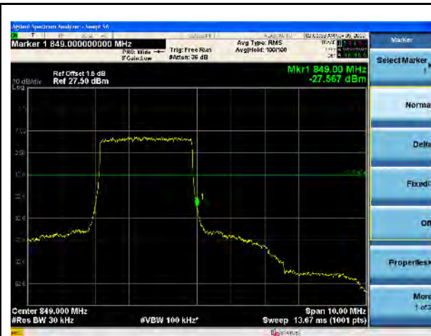
LTE Band 5, QPSK, 3MHz-High CH, 100% RB
