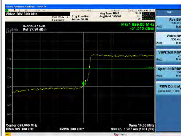
LTE Band 12, 16QAM, 10MHz-Low CH, 100% RB
