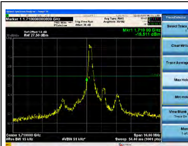
LTE Band 66, QPSK, 1.4MHz-Low CH, 1RB
