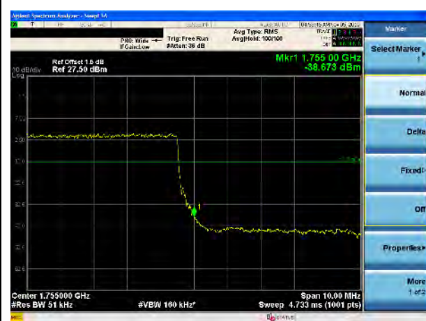
LTE Band 4, 16QAM, 10MHz-High CH, 100% RB
