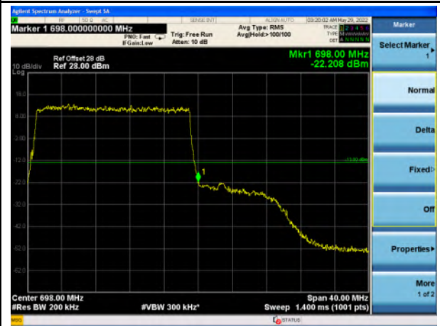
Band 71_QPSK_20M_High_Full RB Config
