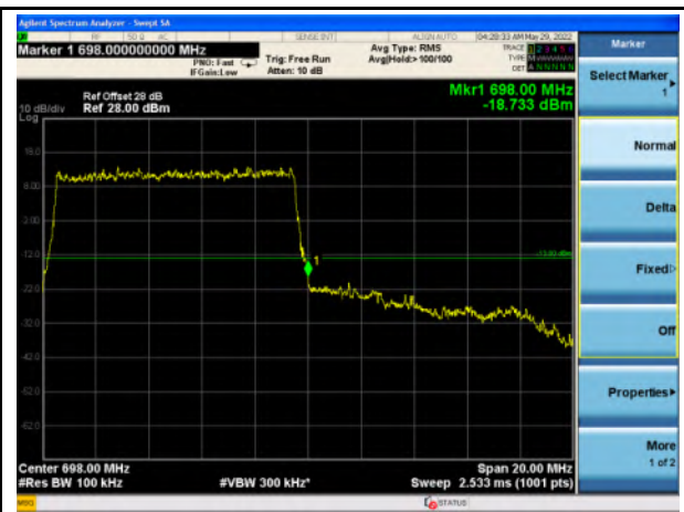
Band 71_QPSK_10M_High_Full RB Config
