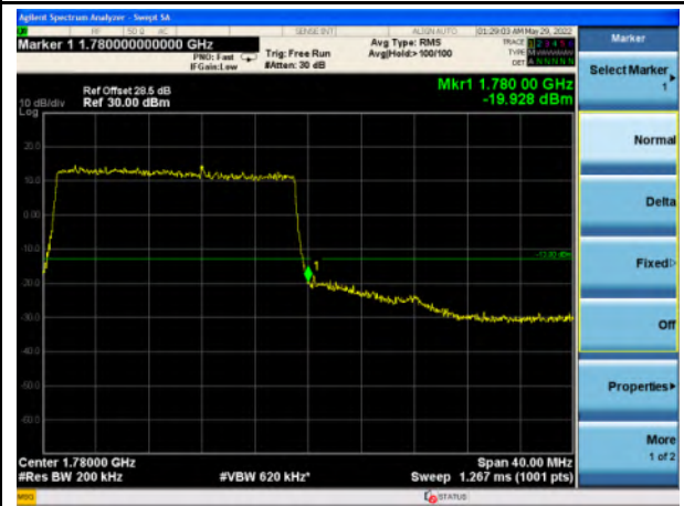
Band 66_QPSK_20M_High_Full RB Config
