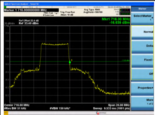
Band 12_QPSK_5M_High_Full RB Config
