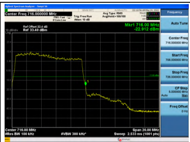
Band 12_QPSK_10M_High_Full RB Config
