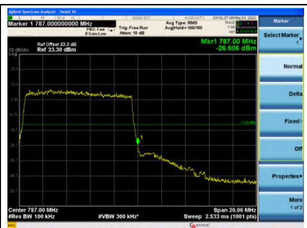
Band 13_QPSK_10M_High_Full RB Config
