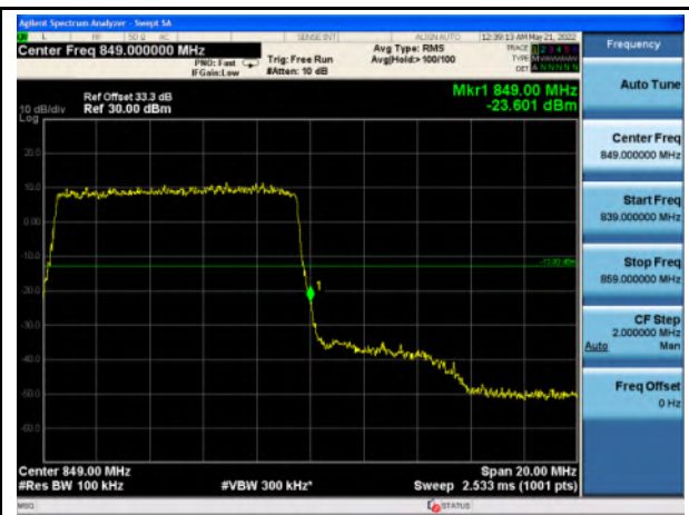
Band 5_QPSK_10M_High_Full RB Config
