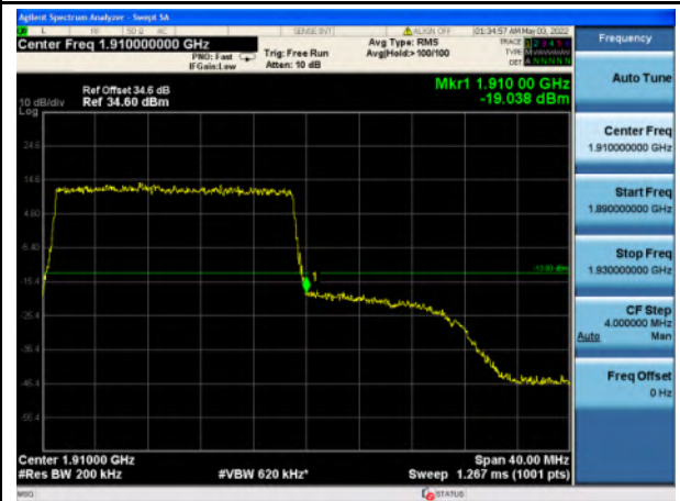
Band 2_QPSK_20M_High_Full RB Config
