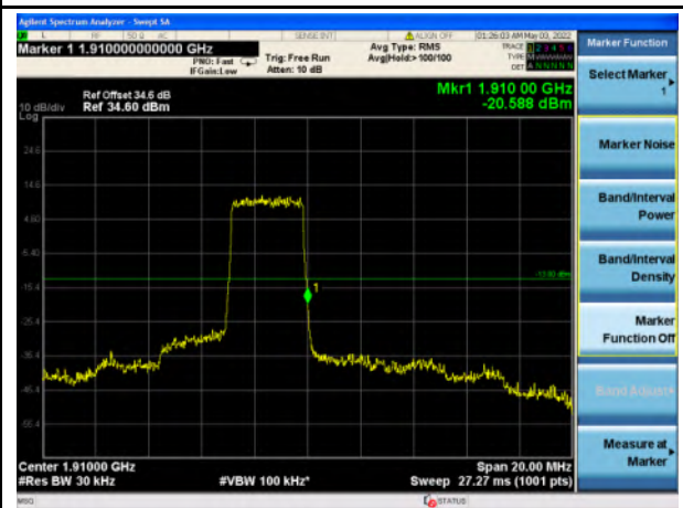
Band 2_QPSK_3M_High_Full RB Config
