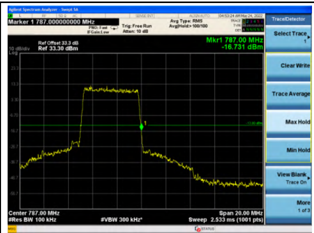
Band 13_QPSK_5M_High_Full RB Config
