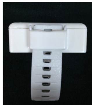
Figure 1.8 Ensure the strap does not go past the top two notches on the latching mechanism.
