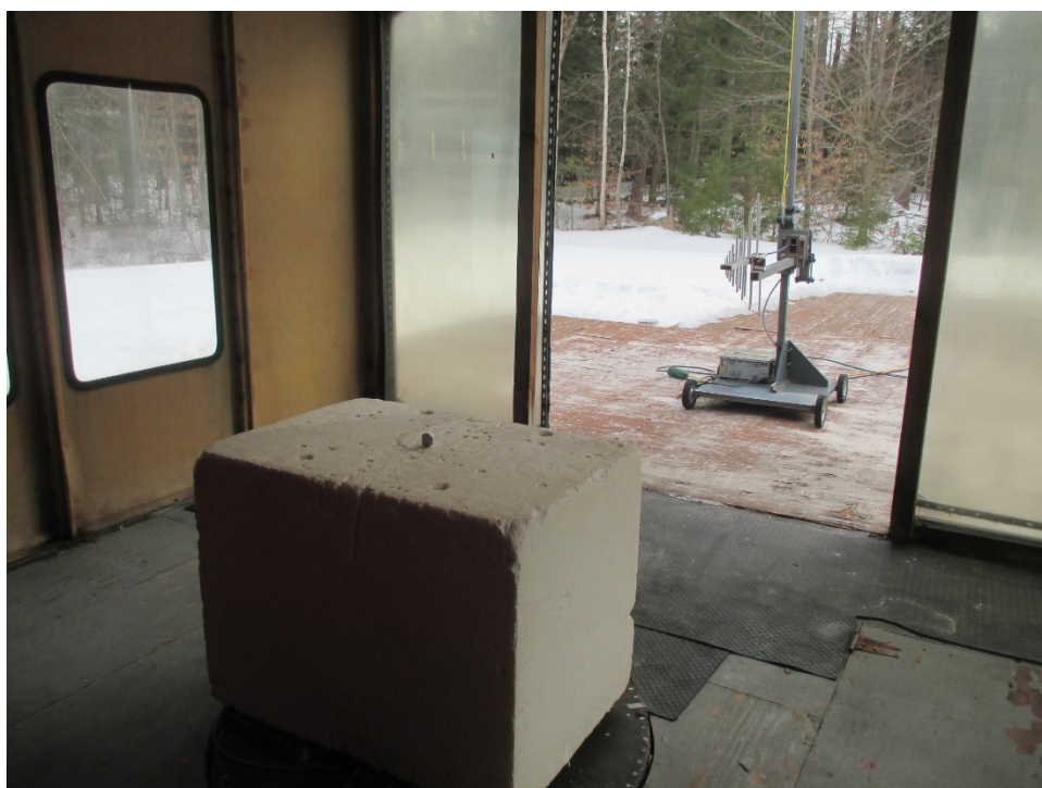
Test Setup, 200 MHz to 1 GHz, Vertical Antenna Polarization
