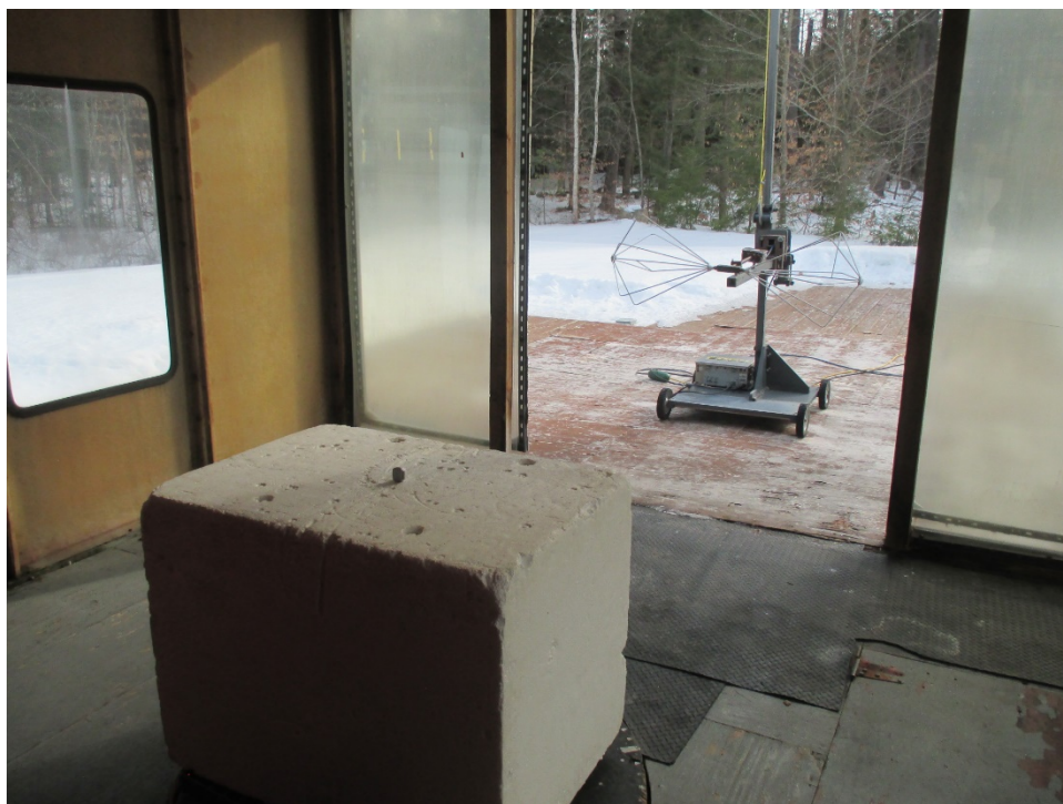
Test Setup, 30 MHz to 200 MHz, Horizontal Antenna Polarization
