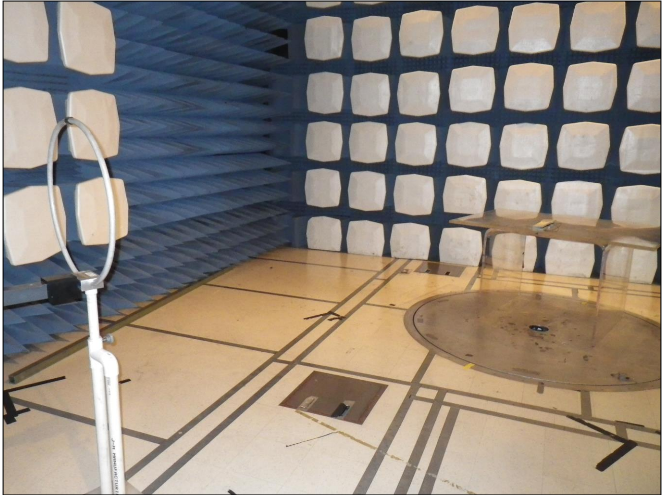
Photograph 3. Transmitter Unit, Field Strength, Test Setup
