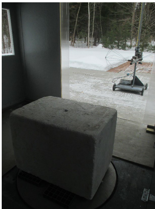
Test Setup, 30 MHz to 200 MHz, Horizontal Antenna Polarization
