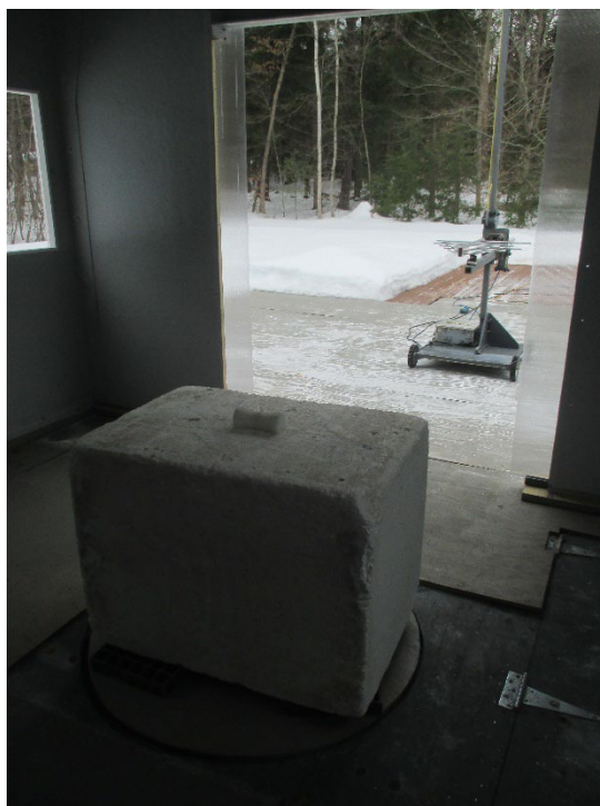
Test Setup, 200 MHz to 1 GHz, Horizontal Antenna Polarization
