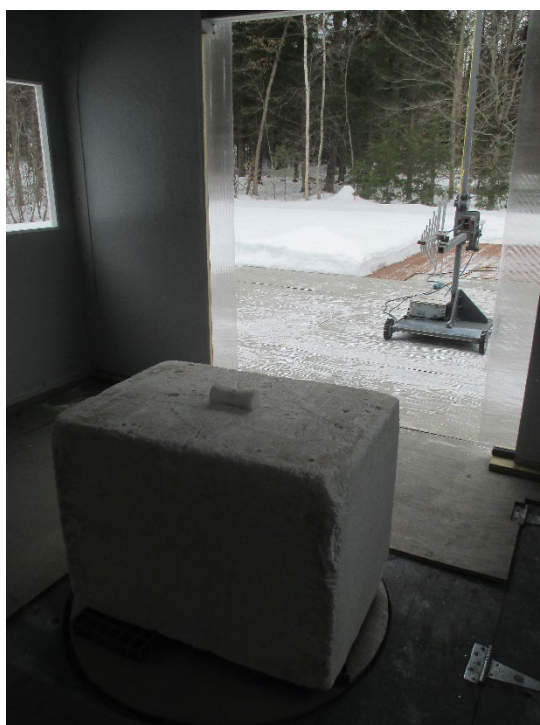
Test Setup, 200 MHz to 1 GHz, Vertical Antenna Polarization
