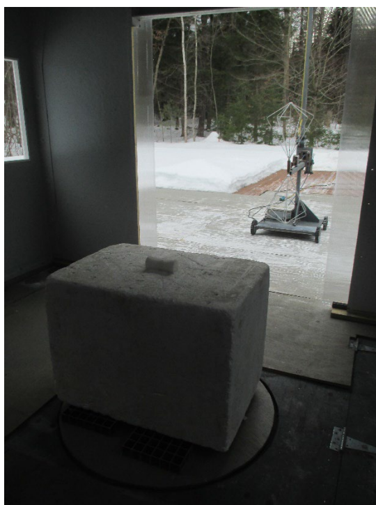
Test Setup, 30 MHz to 200 MHz, Vertical Antenna Polarization
