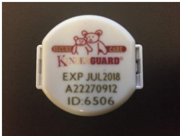
Figure 2-1 13.56 Infant Cutband with STAT ID transmitter
